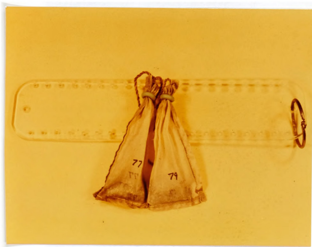
Figure 7. ABOVE: Nylon bags (2000 holes/cm 2 ) were tied to teflon paddle. Elastrator bands were placed over top of bag to insure proper seal of bag. FOLLOWING PAGE: Nylon bag containing known amount of sample was suspended into the rumen of a cammulated steer.
