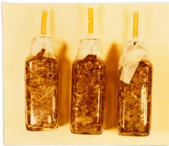
Figure 6. ENSILEMENT STUDY - All biomass species were harvested and packed in triplicate. All samples were gassed with \text{CO}_2 .
