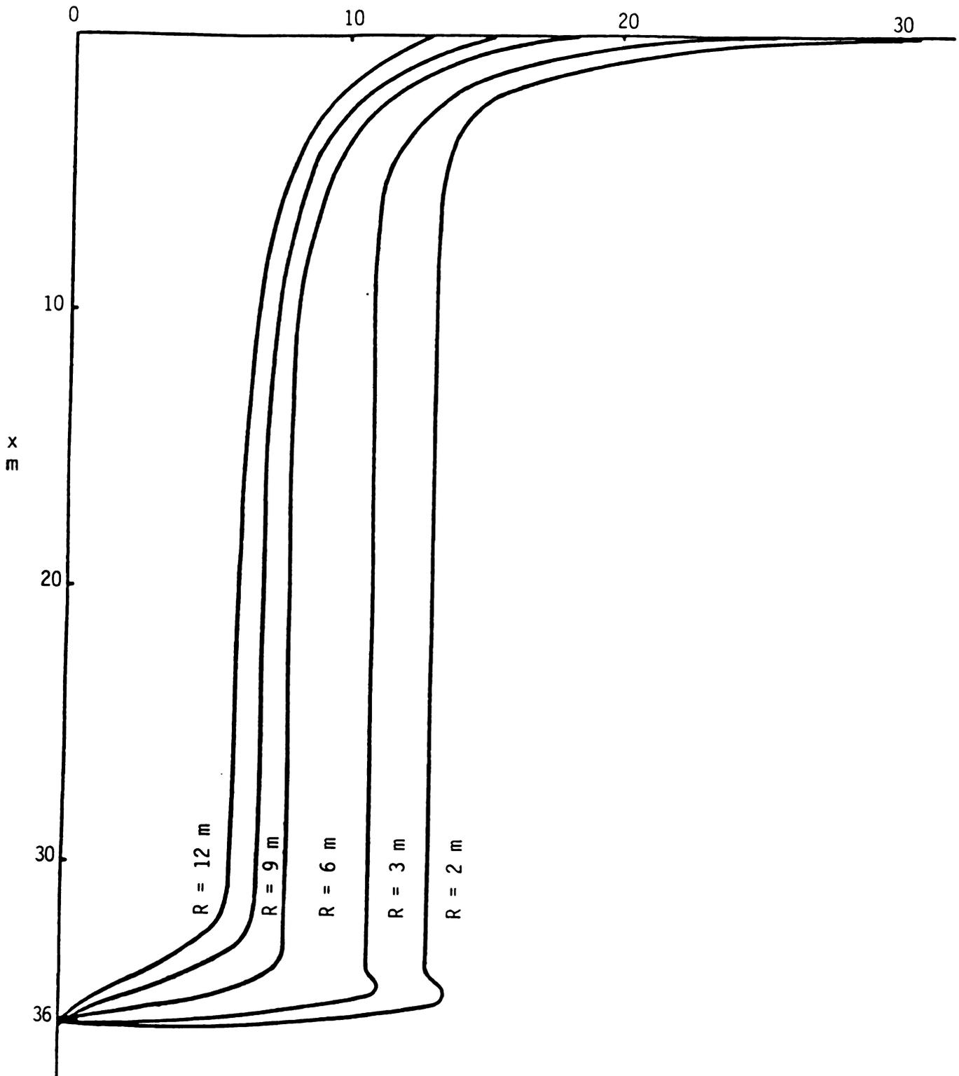
Figure 9. Variation of Percentage Increase in Lateral Pressure due to a Uniform Temperature Drop
