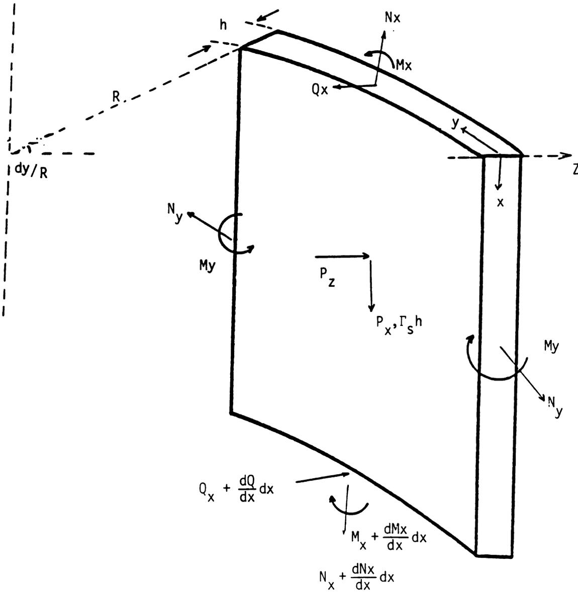
Figure 1. Element of Bin Wall
