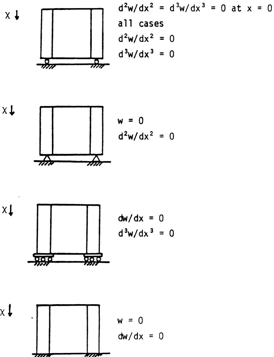
Figure 2. Type of Bottom Edge Restraints
