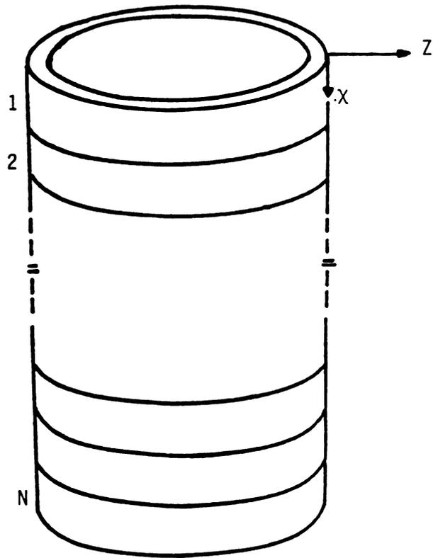
Figure 5. Subdivision of Silo into Small Ring Elements
