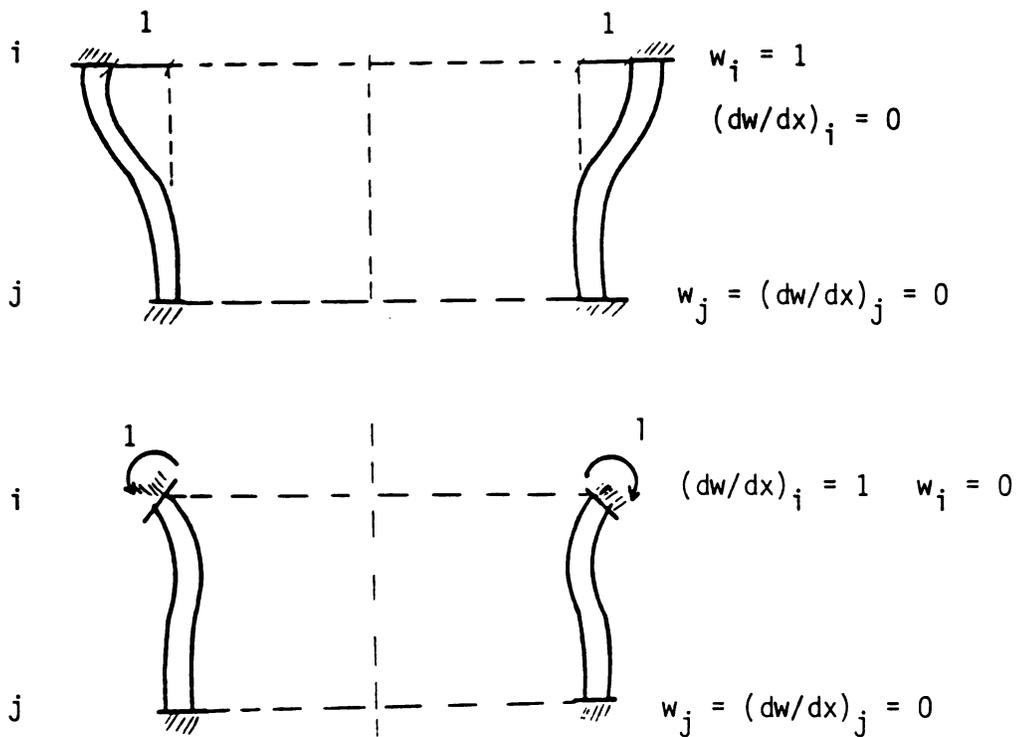
Figure 8. Unit Displacements Load Application to Element Edges
