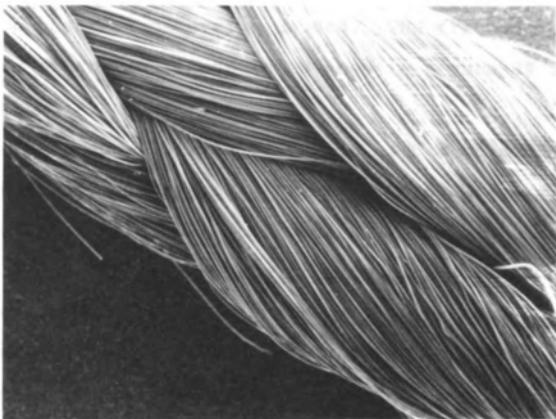
Figure 39. Virgin graphite braid at 50 diameters.
