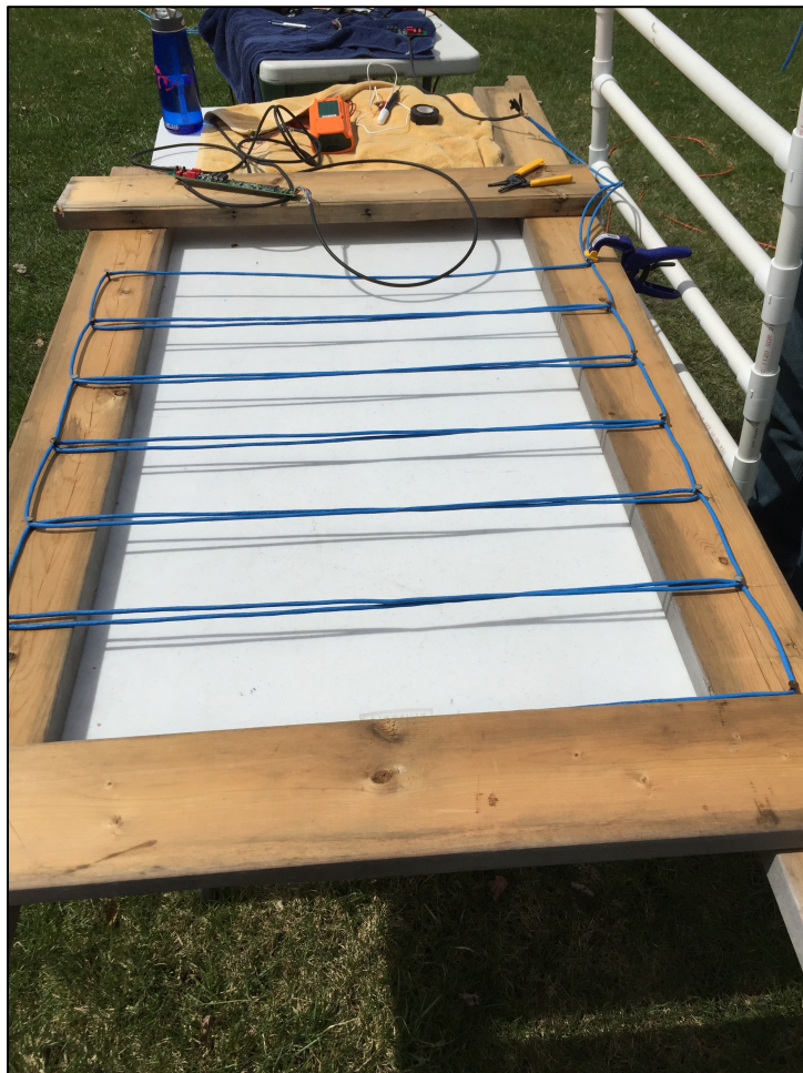
Figure 19. Example of CAT6 ethernet cable wrapped around nails to iteratively test the efficacy varying antenna designs.
