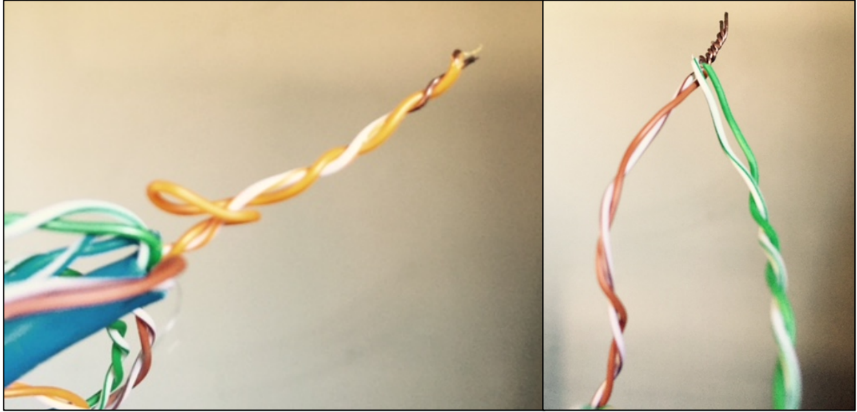
Figure 20. CAT6 Ethernet cable provides four pairs of wire that can be used to produce up to four turns within the antenna structure. The two strands of each color (e.g. solid and striped yellow, left image) should be connected prior to producing loops (shown pre-soldered here). After each end is soldered to its partner, loops can be produced by connecting the ends of two colors (right image).
