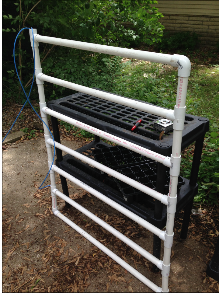
Figure 17. Antenna design for monitoring habitat use of juvenile bluegill sunfish in an experimental pond. The wire loops are made with CAT 6 ethernet cable contained inside PVC tubing. The incorporation of several internal loops was required to accommodate the limited read range for small (7 mm FDX) PIT tags. Each internal loop is 6 inches in height, with total antenna dimensions of 36 in (height) x 32 inches (width).
