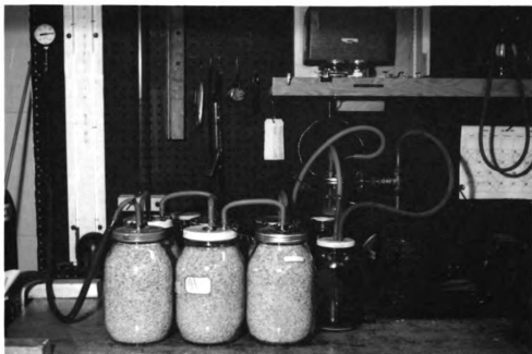
Fig. 5.5--The sealed jars were connected in series through the copper tubings with rubber tubing and the original atmosphere sucked out with a vacuum pump.
