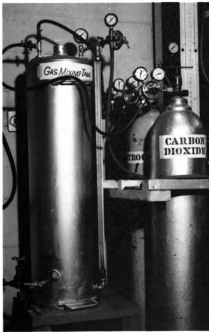
Fig. 5.2--The gas proportions were prepared in a batch mixing tank using water to flood the tank to obtain the different volumes required.
