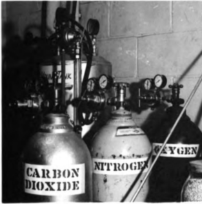
Fig. 5.1--The three main components of air: \text{CO}_2 , \text{N}_2 , and \text{O}_2 were mixed in varying proportions and used as the storage atmosphere in a sealed storage system.
