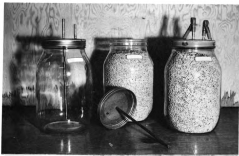
Fig. 5.4--The high moisture grain were stored in hermetically sealed one gallon glass jars whose caps were provided with 3/64 -inch gasket material treated with sealing wax. The caps were fitted with 1/4 -inch copper tubings for introducing the storage gas. The copper tubings were later sealed with rubber tubings and dipped in sealing wax to prevent selective diffusion of carbon dioxide gas.
