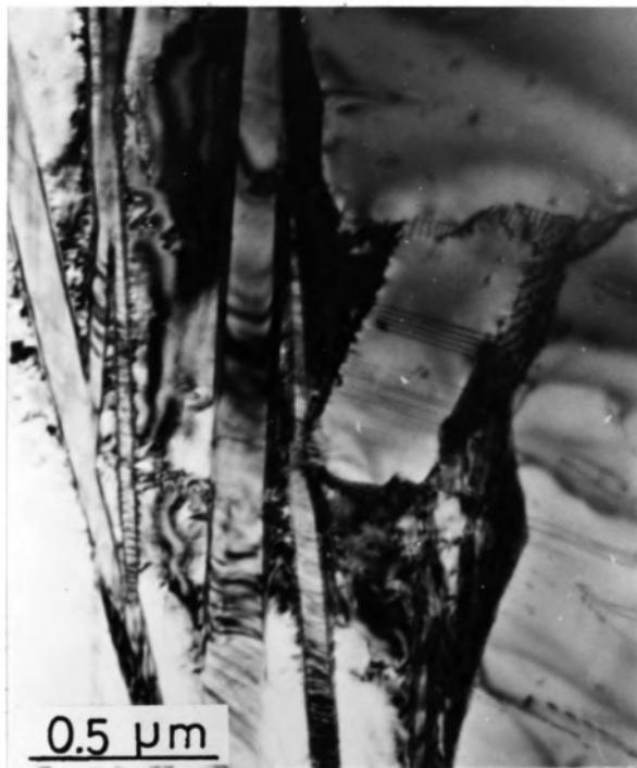
Figure 4.13 High magnification micrograph of a furnace-cooled Ni-14Cu-25Sn specimen, showing many microstructural features.
