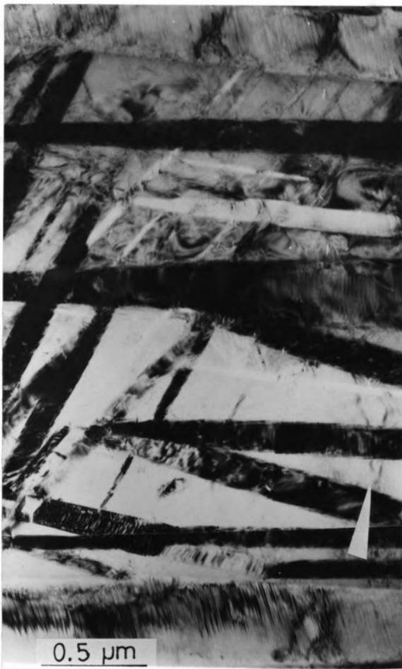
left hand-side of the figure. Here, wide bands coexist with uniformly distributed internal faults. These wide bands formed alternately with dislocated areas. In the dislocated areas, there are small-sized 2H bands showing no internal faults. Some dislocations are also found in internally faulted bands, marked by the double-headed arrow.
