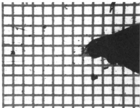
Figure 2.6b A Copper Grating by the Stencil Method.
