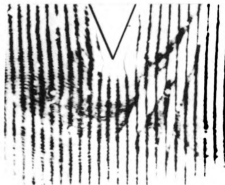
Figure 5.24 The Moiré Fringe Patterns of Loaded and Unloaded on the Quarter Plane of the Notched Specimen in the Direction Parallel to the Crack Line.
