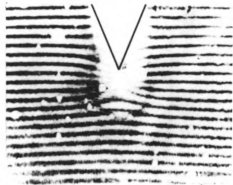
Figure 5.26 The Moiré Fringe Patterns of Unloaded and Loaded on the Quarter Plane of the Notched Specimen in the Direction Parallel to the Crack Line.
