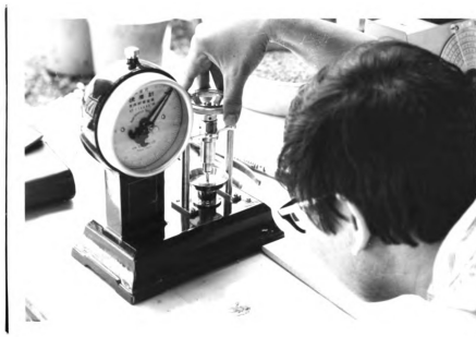
Figure 3.10. Pressure was applied on the grain until it cracked and the force and pressure recorded. A total of 50 grains at each moisture content level was tested.
