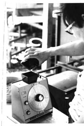
Figure 3.8. Moisture content of samples were measured using a capacitance moisture meter.
