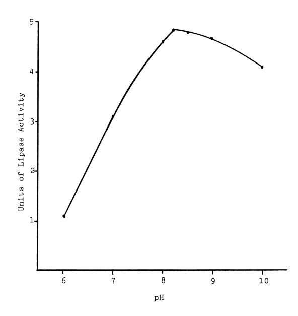
Fig. 8.--Lipase activity on olive oil emulsion as a function of pH during a one hour period.
