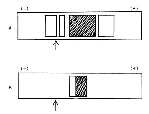
Fig. 11.--The complex electrophoretic pattern (Fig. 11A) on cellulose acetate of the crude lipase fraction II as contrasted with the simple pattern (Fig. 11B) of the final purified fraction IV. The diagonal lines indicate areas of lipase activity.
