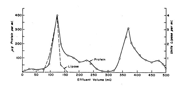
Fig. 3.--Elution pattern of crude lipase (fraction II) preparation from Sephadex G-200. The eluant was 0.1 M Tris (pH 8.0).
