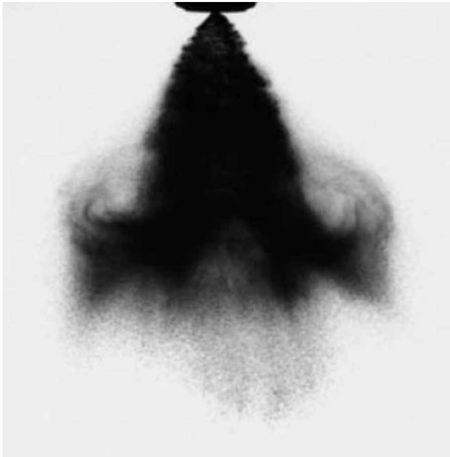
Figure 4.4 Backlit image of a direct Diesel injection spray
