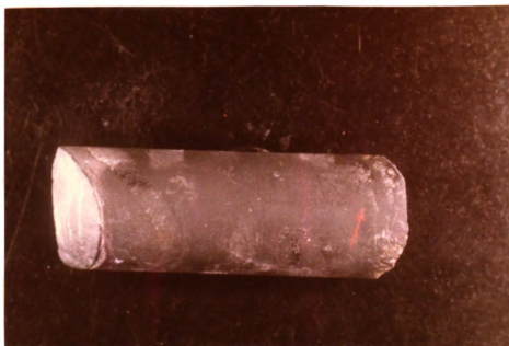
Figure 13. Core segment 2761-4 exhibiting a possible offshoot from the primary layer to the right. Core diameter is 1.9 inches.
