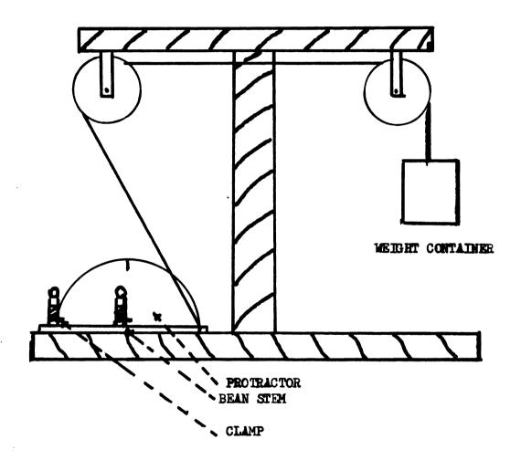
Figure 20 Apparatus to measure strength and resilience of bean stems.
