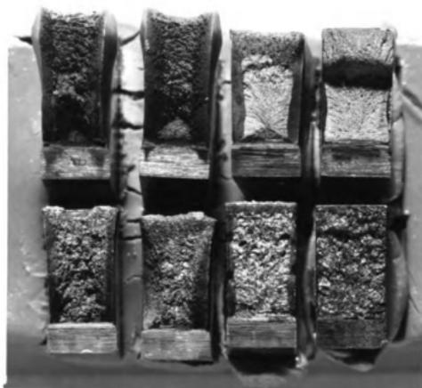
Fig. 46. Fractures of quenched and tempered specimens of Republic #5054025 (IF), AISI 1046. Top row: austenitized 1500°F., 5 min. Bottom row: austenitized 2100°F., 4 hrs. From left to right: fractured at 22°C., -62°C., -114°C., and -196°C.
