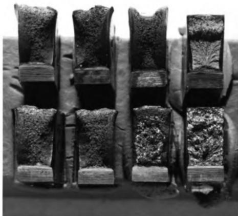
Fig. 44. Fractures of quenched and tempered specimens of Youngstown #95313 (IF), AISI 1040. Top row: austenitized 1500°F., 5 min. Bottom row: austenitized 2100°F., 4 hrs. From left to right: fractured at 22°C., -62°C., -114°C., and -196°C.
