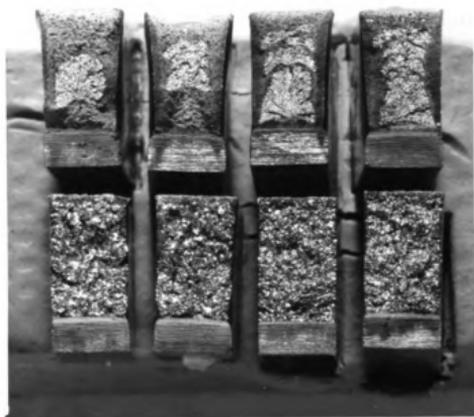
Fig. 47. Fractures of air-cooled specimens tested at 22°C. Top row: air-cooled from fine grained austenite. Bottom row: air-cooled from coarse grained austenite. From left to right: Youngstown #66797 (IC), AISI 1040; Youngstown #95313 (IF), AISI 1040; Republic #5023766 (IC), AISI 1046; Republic #5054025 (IF), AISI 1046.
