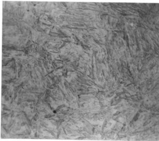
Fig. 16. As-quenched martensite structure for Youngstown #66797 (IC) (AISI 1040) Top: austenitized at 2000°F., 4 hours. Bottom: austenitized at 1500°F., 2 minutes (1000x), nital etch
