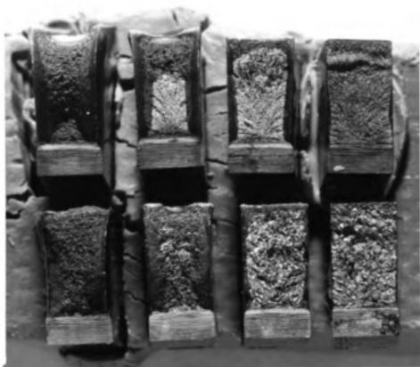
Fig. 45. Fractures of quenched and tempered specimens of Republic #5023766 (IC), AISI 1046. Top row: austenitized 1500°F., 2 min. Bottom row: austenitized 2100°F., 4 hrs. From left to right: fractured at 22°C., -62°C., -114°C., and -196°C.
