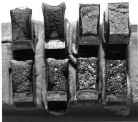
Fig. 43. Fractures of quenched and tempered specimens of Youngstown #66797 (IC), AISI 1040. Top row: austenitized 1500°F., 2 min. Bottom row: austenitized 2000°F., 4 hrs. From left to right: fractured at 22°C., -62°C., -114°C. and -196°C.
