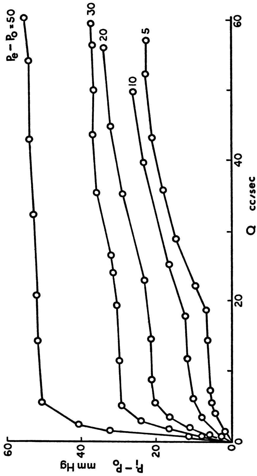
Figure 3. Pressure-flow relationships of 7.5 cm Penrose tubing held at manufactured length during water perfusion.
