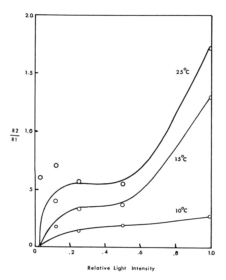
10<sup>-3</sup> M KCl solution. Rl and the ratio of R2 to Rl were plotted against the light intensity as a function of temperature for a given pH gradient.
