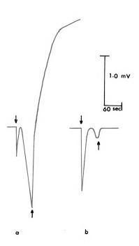
light-off the response slowly recovered the original base line and never passed over it, unlike the response shown in Figure 33a. These two types of photoresponses following a long time illumination are very important in elucidating the mechanism of generation of the photopotentials.
