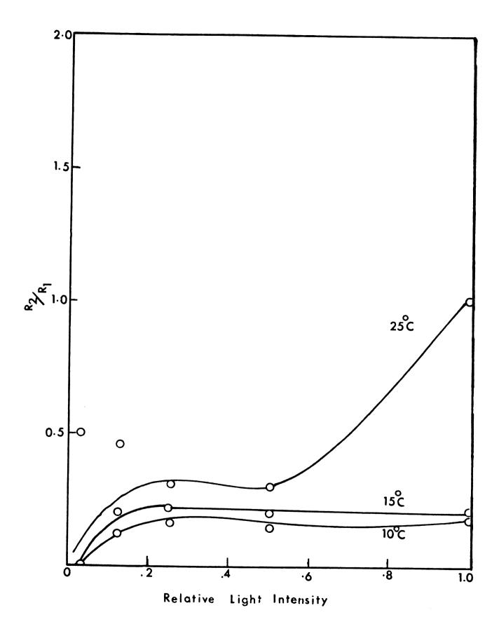
Figure 18.--The effect of relative intensity of light on R2/R1 at  $\Delta$ pH 2.0 as a function of temperature. The inner pH was 3.3 and the outer pH was higher. The inner chamber contained about  $10^{-3}$  M FeCl $_3$  in  $10^{-3}$  M KCl while the outer chamber contained HCl and the same concentration of KCl.
