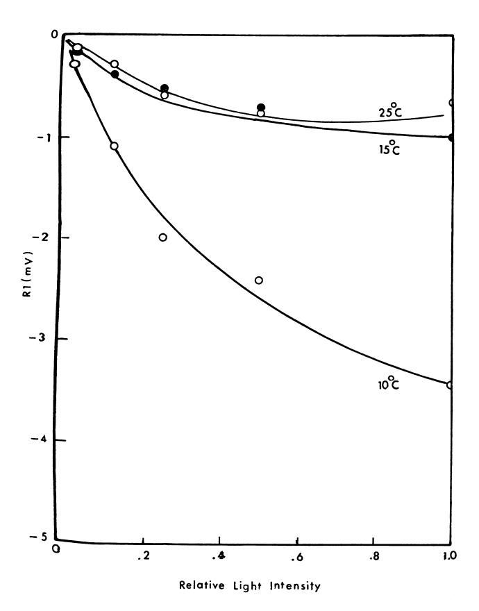
Figure 15.--The effect of relative intensity of light on R2/R1 at  $\Delta$ pH 0.3 as a function of temperature. The inner pH was 3.3 and the outer pH was higher. The inner chamber contained about  $10^{-3}$  M FeCl $_3$  in  $10^{-3}$  M KCl while the outer chamber contained HCl and the same concentration of KCl.
