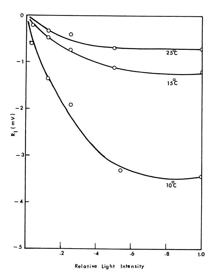
Figure 14.--The effect of relative intensity of light on Rl component at  $\Delta pH$  2.0 as a function of temperature. The inner pH was 3.3 and the outer pH was higher. The inner chamber contained about  $10^{-3}$  M FeCl $_3$  in  $10^{-3}$  M KCl while the outer chamber contained HCl and the same concentration of KCl.
