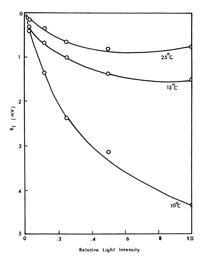
Figure 13.--The effect of relative intensity of light on Rl component at  $\Delta pH$  1.0 as a function of temperature. The inner pH was 3.3 and the outer pH was higher. The inner chamber contained about  $10^{-3}$  M FeCl $_3$  in  $10^{-3}$  M KCl while the outer chamber contained HCl and the same concentration of KCl.
