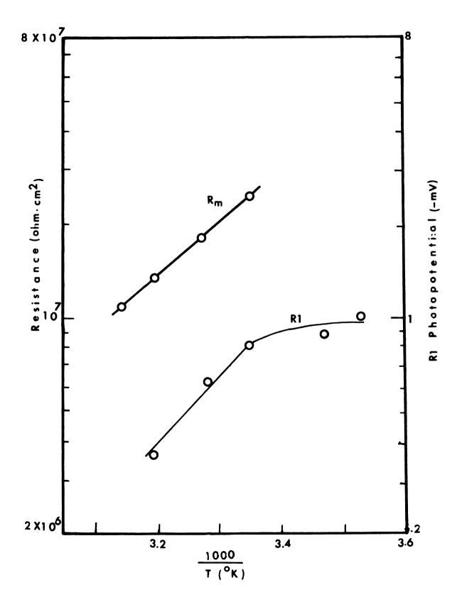
Figure 26.--Dark membrane resistance and Rl
