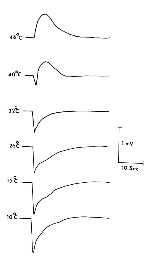
Figure 23.--The time course of the photoresponses of all-trans-retinal BLM as a function of temperature: FeCl<sub>3</sub> system. The aqueous phases contained only HCl with the outside pH at 3.5. The inside chamber contained, in addition to HCl, FeCl<sub>3</sub> to lower pH to 2.8. The duration of the illumination was 1 second.
