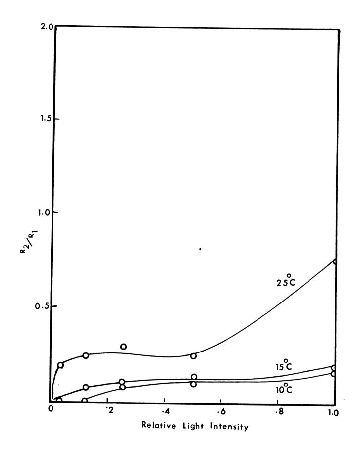
Figure 17.--The effect of relative intensity of light on R2/R1 at  $\Delta$ pH 1.0 as a function of temperature. The inner pH was 3.3 and the outer pH was higher. The inner chamber contained about  $10^{-3}$  M FeCl $_3$  in  $10^{-3}$  M KCl while the outer chamber contained HCl and the same concentration of KCl.
