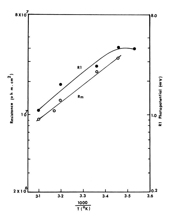
Figure 27.--The relationship between two components of photopotentials and dark membrane resistance.
