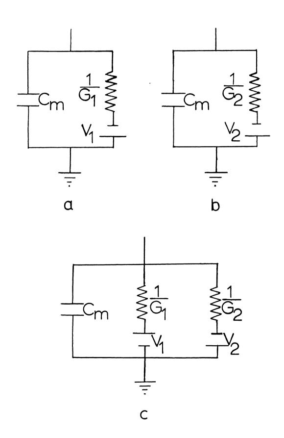
$$v_{c}^{\text{total}} - v_{o} = \frac{G_{1}}{G_{1} + G_{2}} (v_{1} - v_{o}) (1 - e^{-G_{1}t/C_{m}})$$
