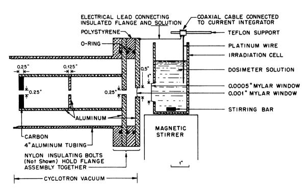
Figure 2. Experimental Arrangement Used for the Collection of Beam Currents from the 86-Inch Cyclotron.
