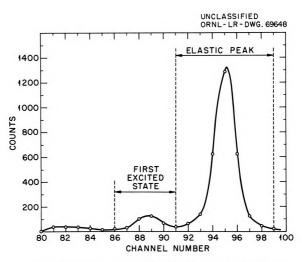
Figure 5. Portion of Nickel Scintillation Spectrum Used in Beam Current Measurement Procedure.
