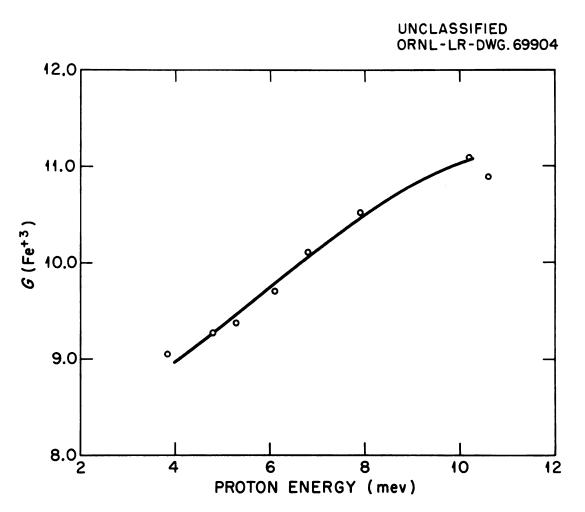
Figure 6. Known Ferric Ion Yields versus Proton Energy (See Reference 3).
