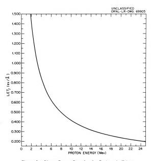
Figure 1. Linear Energy Transfer for Protons in Water.
