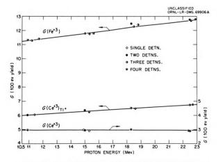
Figure 8. Experimental Yields in the Proton Radiolysis of Ferrous and Ceric Solutions.
