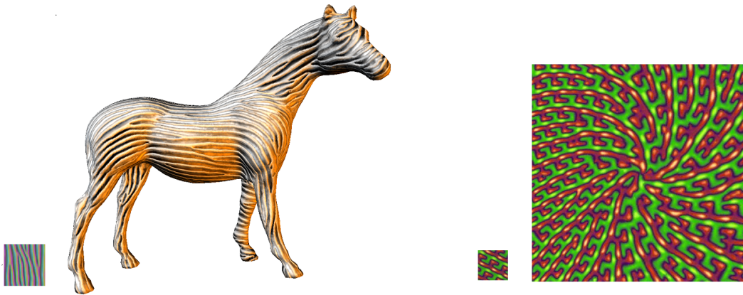
Figure 1.2 Example-based texture synthesis on surface and plane [2]. The square tiles show exemplars that are used to synthesize a texture on surfaces guided by precomputed vector fields.
