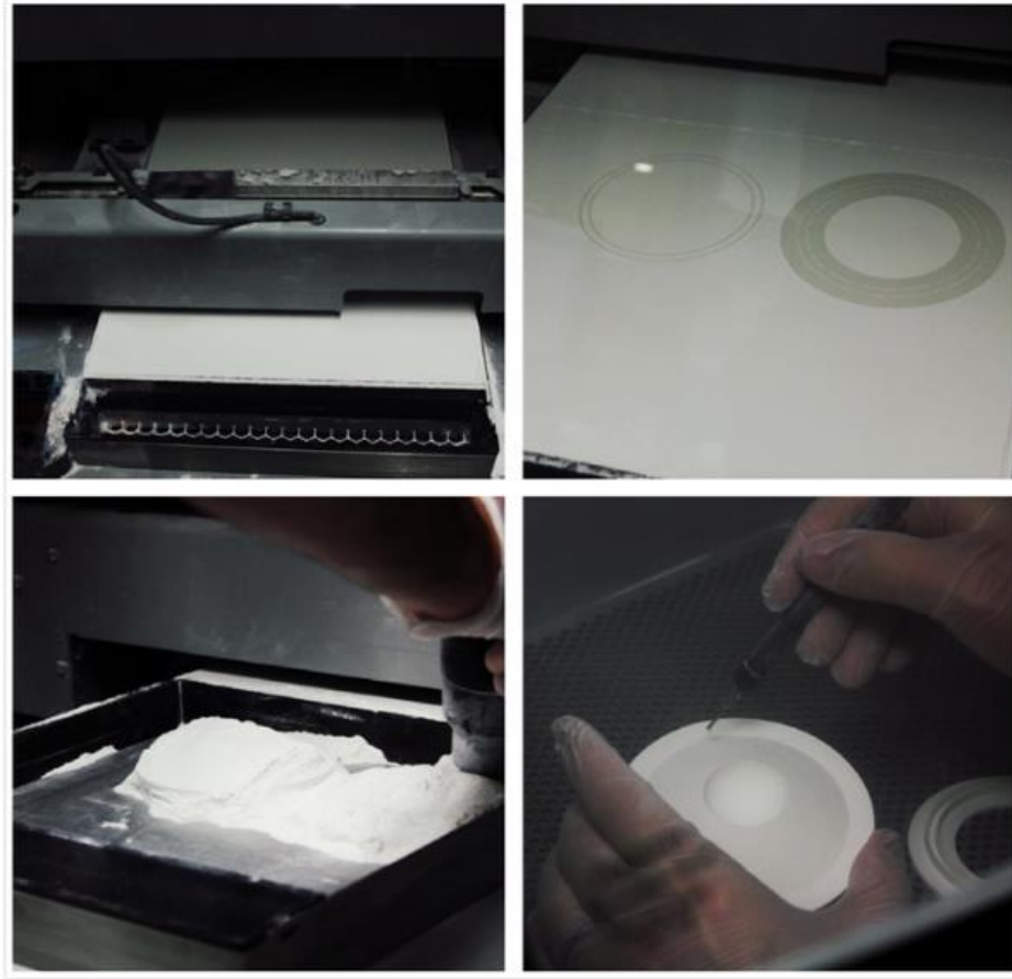
Figure 3-11: Representative images of the 3D printing of loading fixture.
