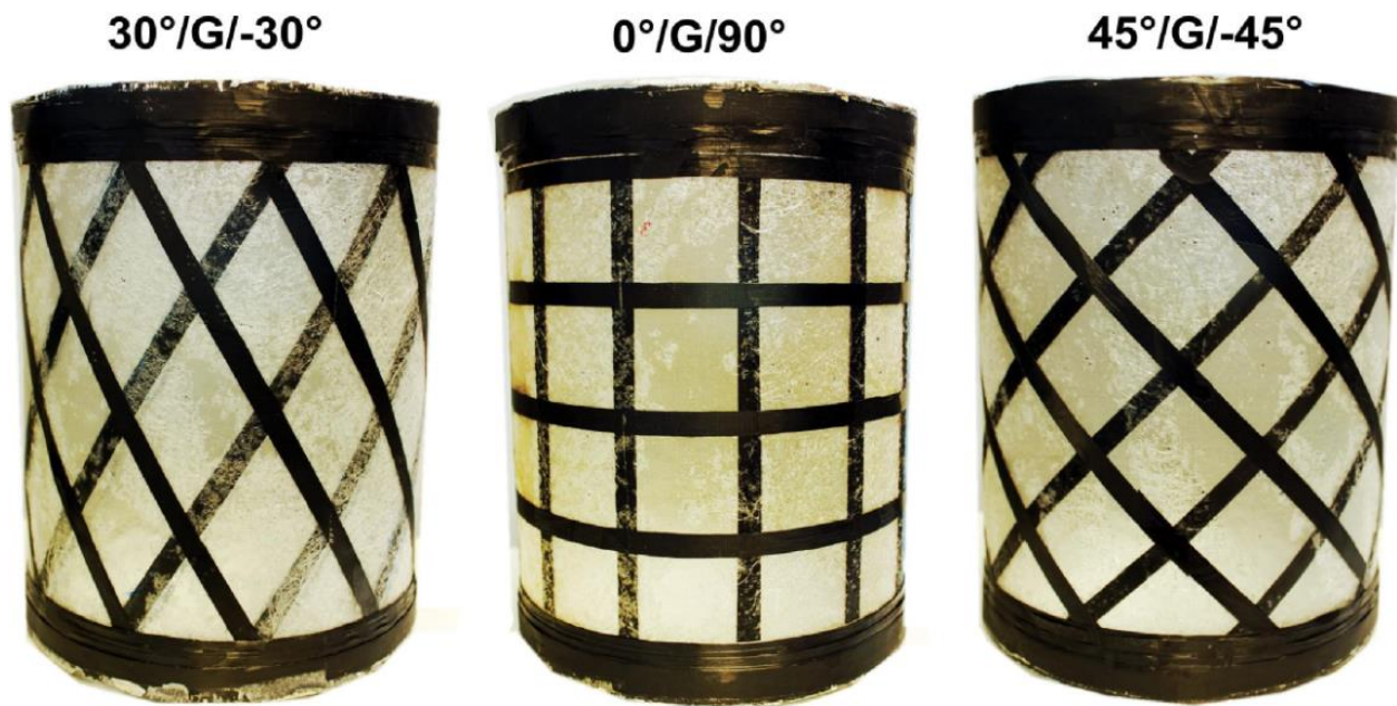
Figure 5-2: Hybrid cylinders with patterned material distributions.
