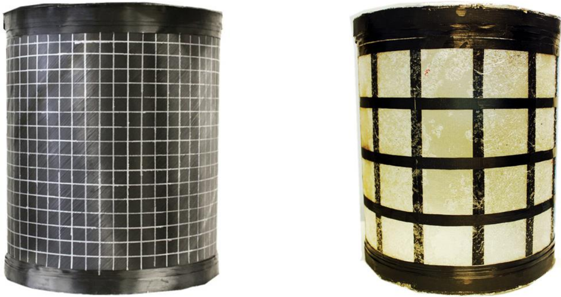
Figure 3-3: Carbon/epoxy cylinder (left) and hybrid carbon/E-glass/epoxy cylinder (right).
