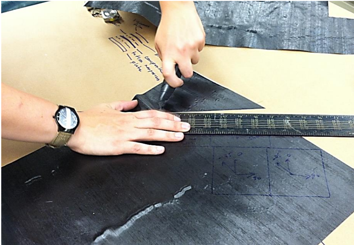
Figure 3-6: The cutting of CFRP prepregs.
