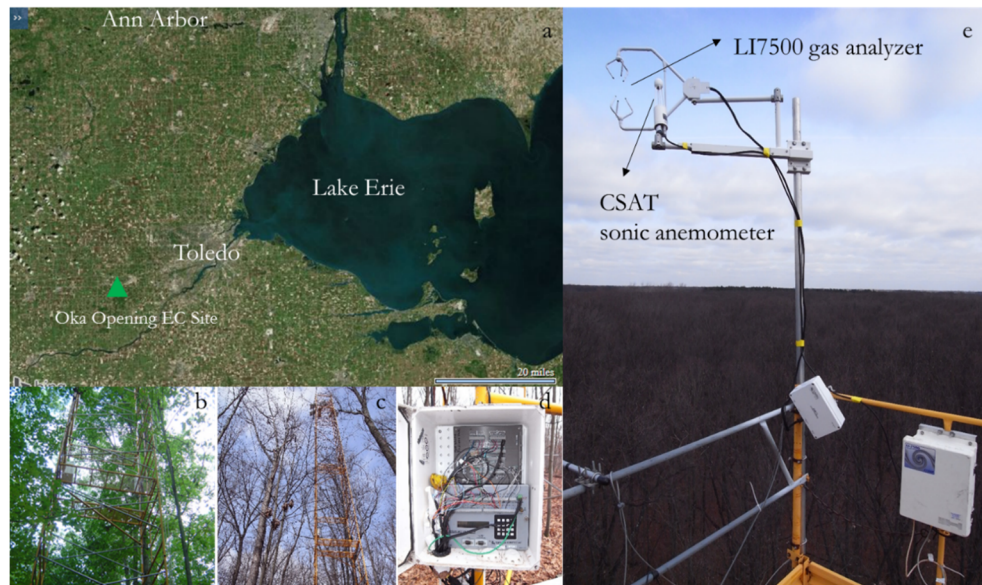
Figure 2.1, The location of the study site (a), side views of the EC tower in both summer (b) and winter (c) , the CR5000 data collection logger (d), and EC systems (LI-7500 and CSAT3, e)
