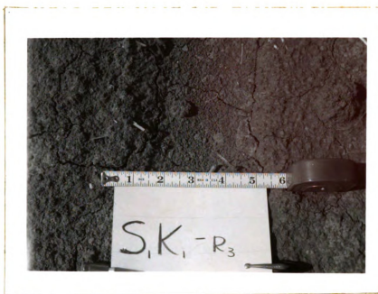
Fig. 13. Crusting of Brookston clay loam processed at 1600 rpm and treated with 0.1 percent Krilium
