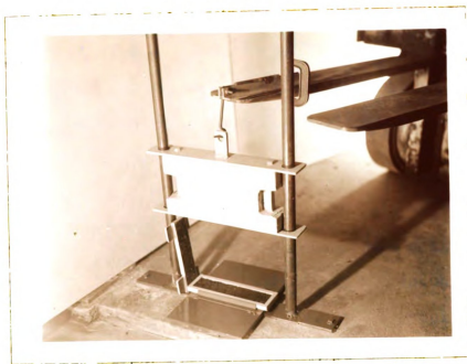
Fig. 19. Impact device for mechanically treating soil to devitalize the entrained weed seeds
