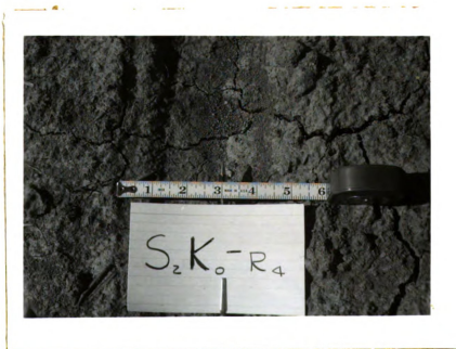
Fig. 12. Crusting of Brookston clay loam on row processed at 2600 rpm and approximately one inch deep
