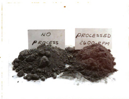
Fig. 30. Soil structure damage immediately after processing
