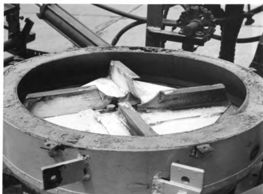
Fig. 22. Redesigned impeller and impact plate
