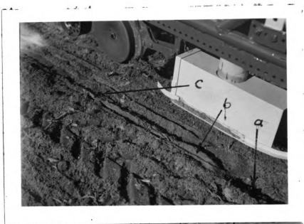
Fig. 9. Close-up view of the right-hand side of the planter lifted up to show the processed strip of soil
