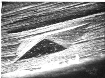
FIGURE 5 NEGATIVE REPLICA OF INDENTATIONS
