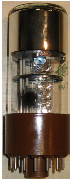
Figure 2.12 An example of a photomultiplier [13].
