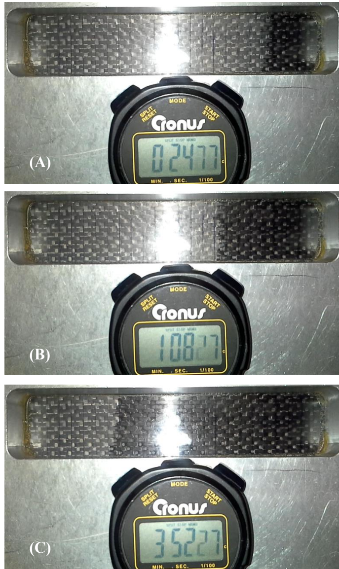
Figure 5.10: Linear Flow Front Advancement through Non-Tackified IM7-4HS. (A) Flow front at 24 sec. (B) Flow front at 1 min. 8 sec (C) Flow front at 3 min. 52 sec.
