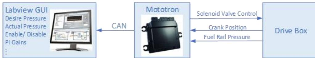
Figure 3: Fuel Rail System Control Block Diagram
