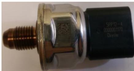
Figure 11: Chrysler Fuel Sensor
