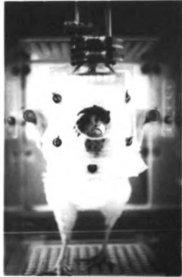
Figure 4.6-- Chicken position in the calorimeter
