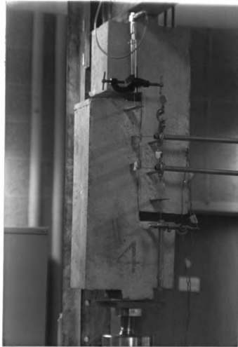
Figure 3.12: Test Set-Up For Dowel Action Against Core.
