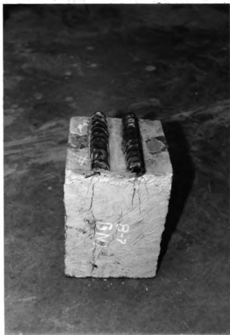
Figure 3.6: Split Cracking of Multiple Bar Specimen.
