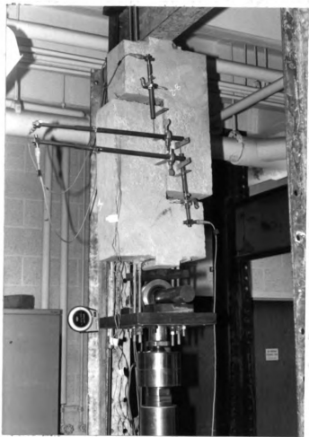
Figure 3.23: Test Set-Up For Dowel Action Against Cover.
