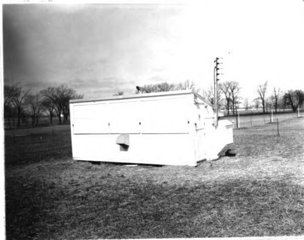
Figure 5. The house with no glass area. This house, converted from the one-half double pane house, was used in the fourth and subsequent trials.
