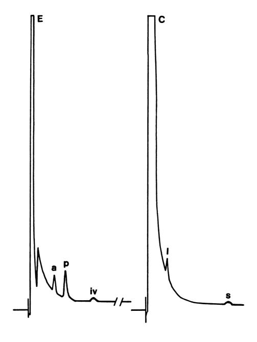
Fig. 15. A gas chromatogram showing the volatile (left) and non-volatile (right) acid end products of  $\underline{B}$ . clostridiiformis ss clostridiiformis (23a). For explanation of symbols, refer to  $\underline{p}$ .  $\underline{x}$ .
