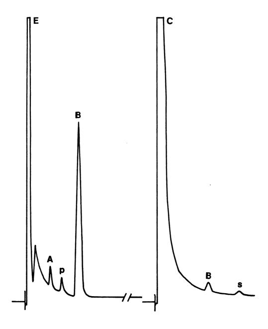
Fig. 18. A gas chromatogram showing the volatile (left) and non-volatile (right) acid end products of  $\underline{F}$ . necrophorum (#27). For explanation of symbols, refer to  $\underline{p}$ .  $\underline{x}$ .
