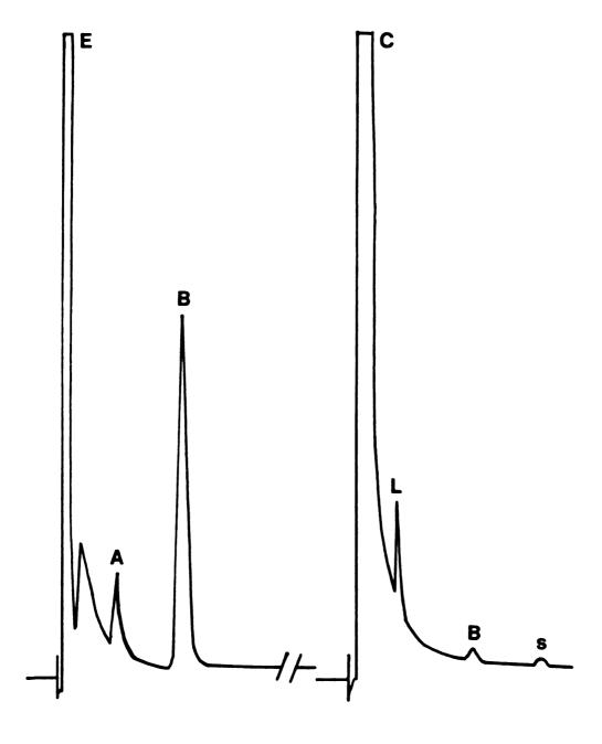
Fig. 11. A gas chromatogram showing the volatile (left) and non-volatile (right) acid end products of  $\underline{C}$ . beijerinckii (#34). For explanation of symbols, refer to p. x.
