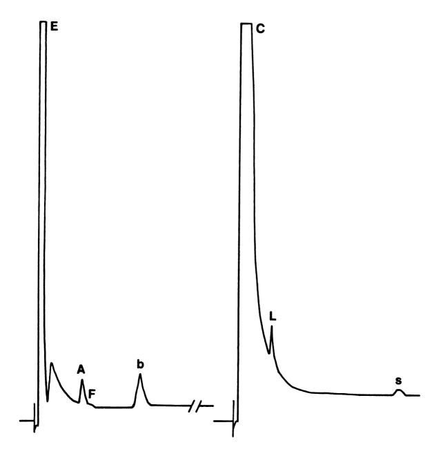
Fig. 8. A gas chromatogram showing the volatile (left) and non-volatile (right) acid end products of  $\underline{C}$ .  $\underline{tertium}$  (#44b). For explanation of symbols, refer to  $\underline{p}$ .  $\underline{x}$ .
