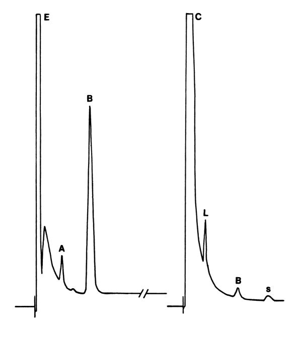
Fig. 5. A gas chromatogram showing the volatile (left) and non-volatile (right) acid end products of  $\underline{C}$ .  $\underline{barati}$  (#26c). For explanation of symbols, refer to p. x.
