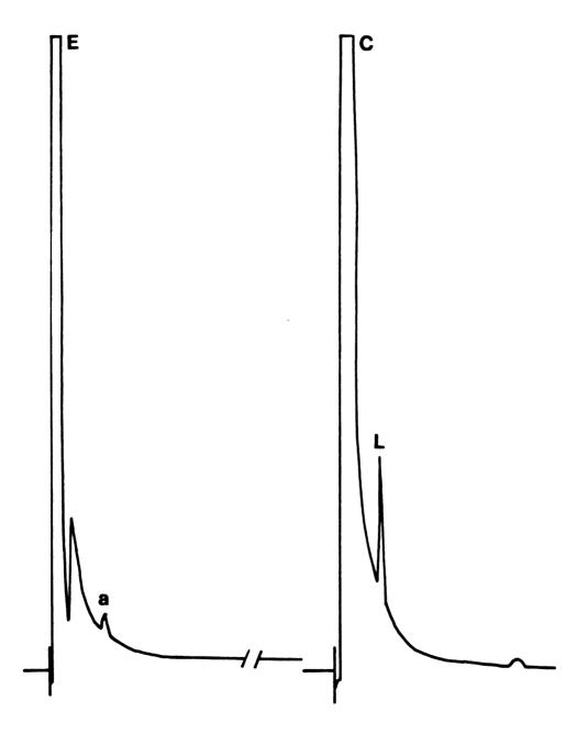
Fig. 12. A gas chromatogram showing the volatile (left) and non-volatile (right) acid end products of  $\underline{C}$ .  $\underline{ramosum}$  (#37b). For explanation of symbols, refer to  $\underline{p}$ .  $\underline{x}$ .
