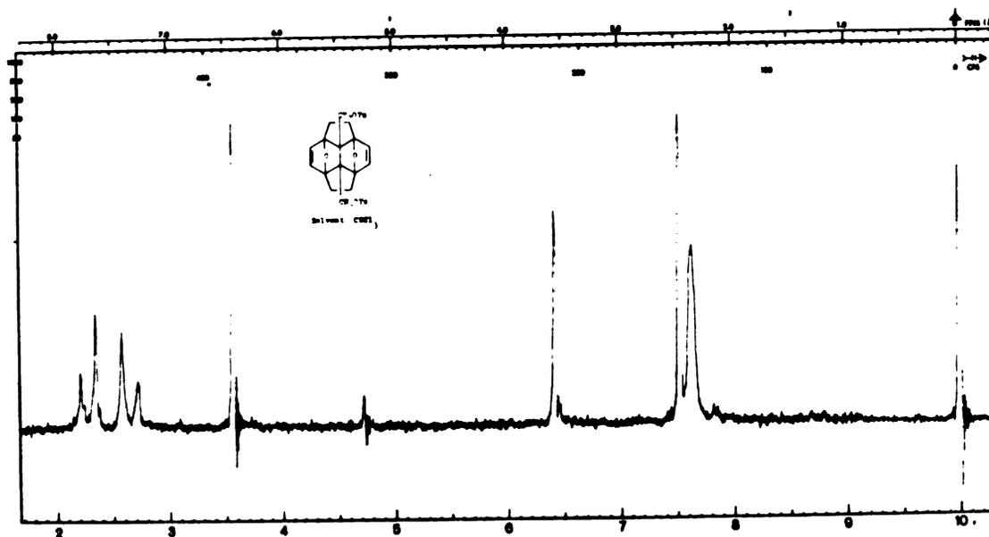
Figure 21. Nmr spectrum of ditosylate 16.
