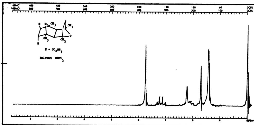
Figure 33. Nmr spectrum of trans-diester 73.
