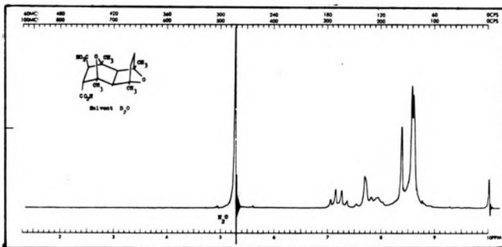
Figure 28. Nmr spectrum of diacid 50.
