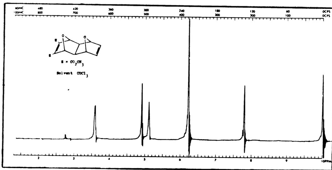
Figure 39. Nmr spectrum of adduct 37.
