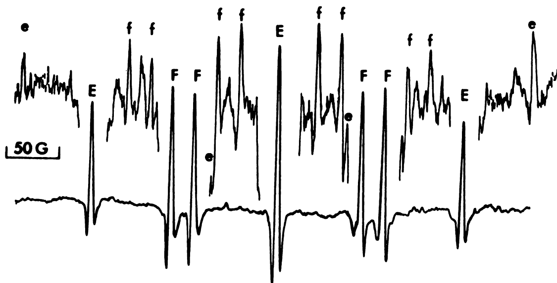
Figure 22a. Second-derivative ESR spectrum of the radicals produced in single crystals of ammonium difluoroacetate irradiated at room temperature. The direction of the magnetic field is parallel to c . The gain has been increased by 1000 to permit observation of the ^{13}\text{C} satellites since the natural abundance of ^{13}\text{C} is only 1.1%.
