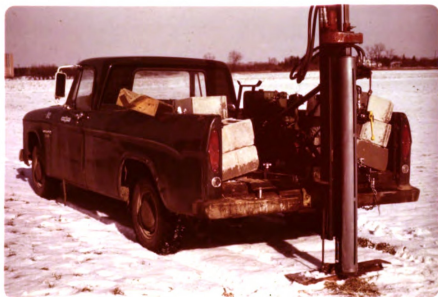
Figure 16. Hydraulic soil-coring machine with a quick release bit on the end of a 11 x 152 cm soil tube.
