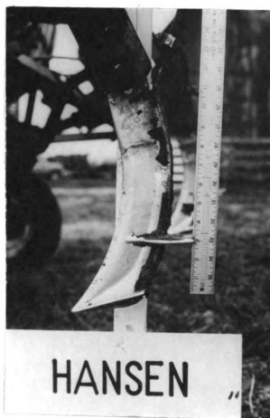
Figure 2. Vertical knife designed for anhydrous ammonia application to grass. The horizontal curved plate, designed by C. M. Hansen, Department of Agricultural Engineering, was welded to the commercial vertical knife to keep \text{NH}_3 loss to a minimum.
