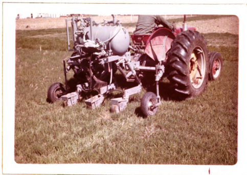
Figure 1. Anhydrous ammonia applicator with three vertical knives.
