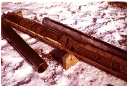
Figure 17. Typical soil profile shown with 9 and 11 cm diameter soil tubes and a measuring trough used to divide the profile into 15-cm increments.
