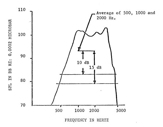
Figure 12. Illustration of frequency range as measured by the HAIC Method and the new method. The frequency response curves obtained from both methods have been superimposed for this illustration.
