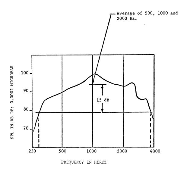
Figure 3. HAIC Method for determining the basic frequency response curve and frequency range of a hearing aid.
