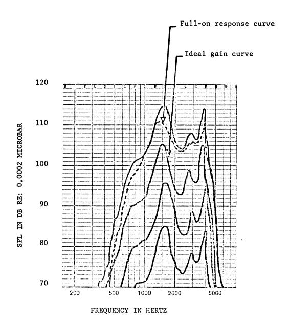
Figure 1. Family of gain curves for a specific hearing aid obtained with a different procedure than advocated by HAIC. A reducation in output is also shown for the full-on volume control adjustment.
