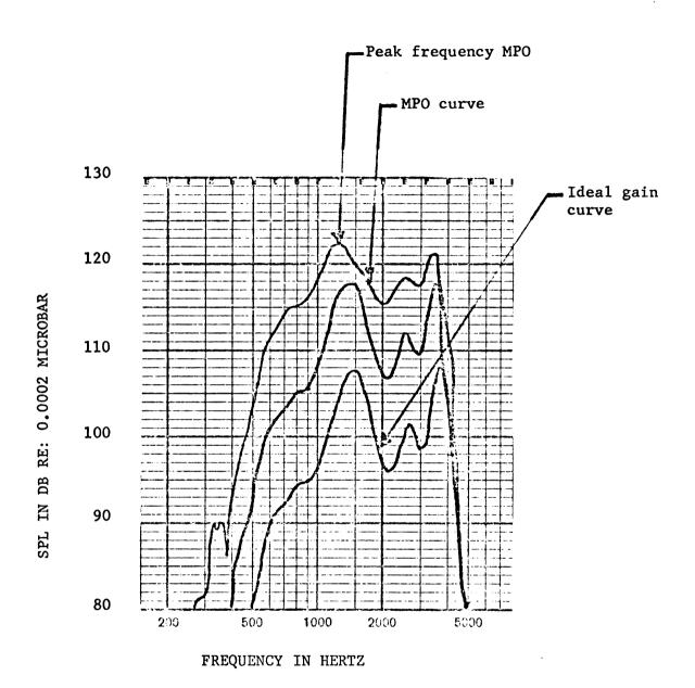
Figure 2. Illustration of the new procedure for determining the maximum power output (MPO) of a hearing aid.
