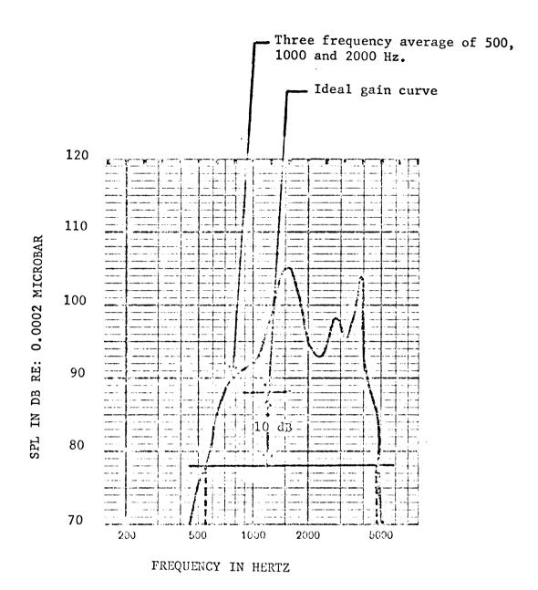
Figure 4. Illustration of proposed method for determining the frequency range of a hearing aid.
