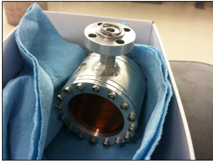
Figure 3.5: (Left) Photo of the target cell used to contain the Liquid Deuterium. The liquid drips down through the center hole seen on the target flange. The iridium seal can be seen surrounding it before being pressed. (Right) Drawing of the inner ring where the Kapton foil is glued. The ring is then clamped to the target by an outer ring visible in the left photo.
