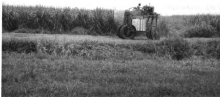
Figure 23. Self-propelled spraying machine. This piece of equipment is especially designed and manufactured for use in cane culture. The machine straddles a row of cane as it applies spray. New machinery made farming more efficient and helped increase yields of cane during 1960-1972.
