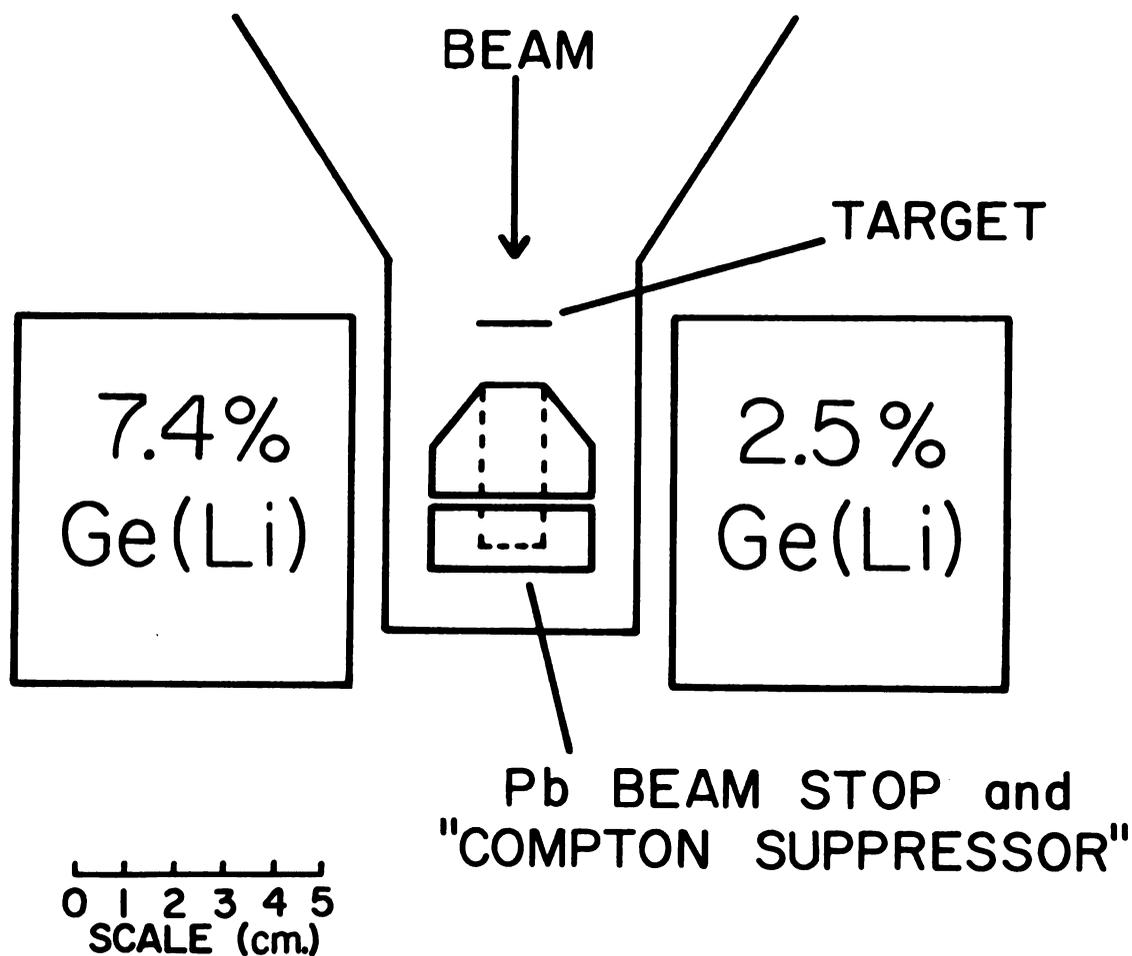
Figure 4. Geometry for the in-beam  $\gamma$ - $\gamma$  coincidence measurements. The squares are not meant to represent the actual size of the Ge(Li) detectors, but only the approximate location of their cryostat caps.
