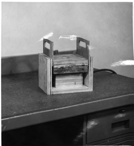
Figure 9. Press device assembled and ready for use. Medium support fixture is hidden by front of plywood slide. Pressure applied by dead load added to top of Carver press platen.
