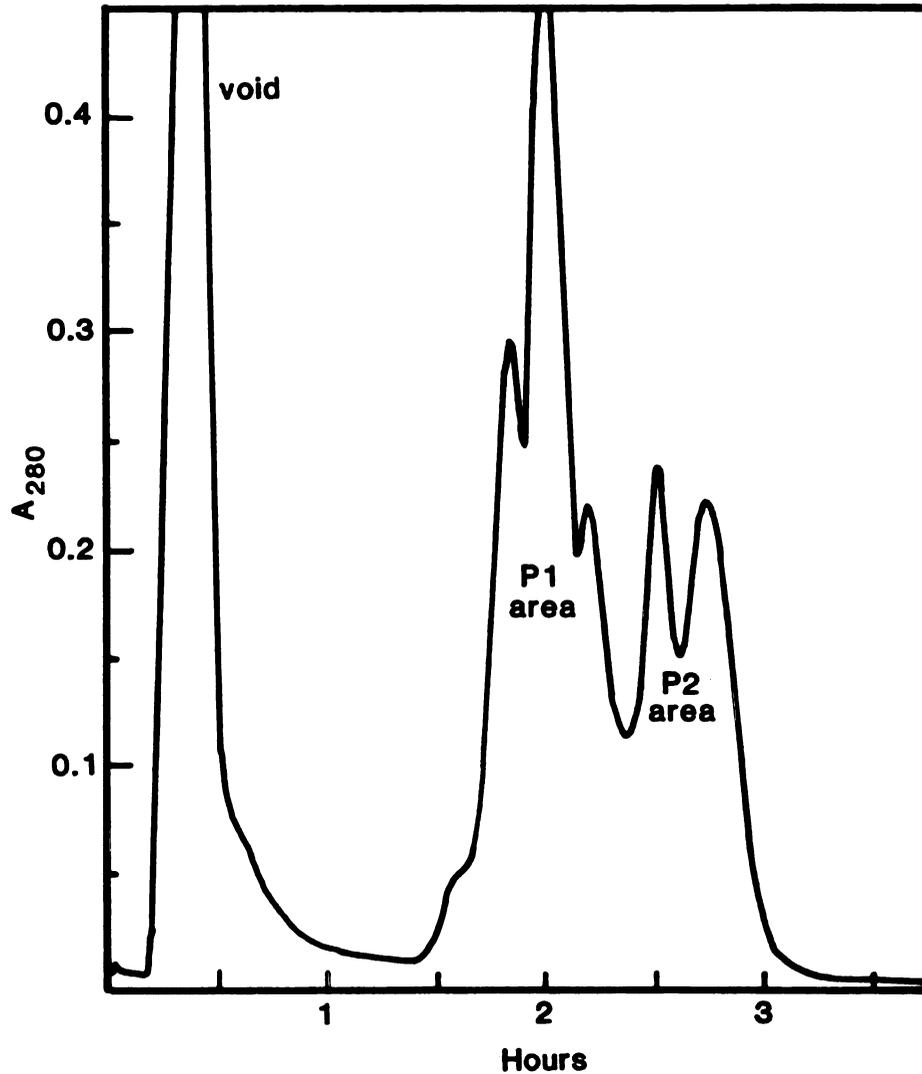
Figure 10. Profile of crude  $\text{CaCl}_2$  eluate before TCA precipitation as separated on carboxymethyl cellulose.
