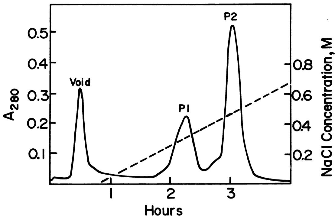
Figure 6. Separation of TCA-precipitated crude HRGP on carboxymethyl cellulose (CM-52), giving P1 and P2.
