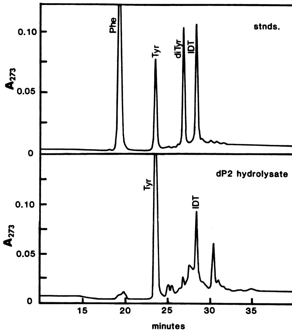
Figure 14. Quantitation of isodityrosine in deglycosylated P2: HPLC separation of a dP2 acid hydrolysate on Hamilton PRP-1.
