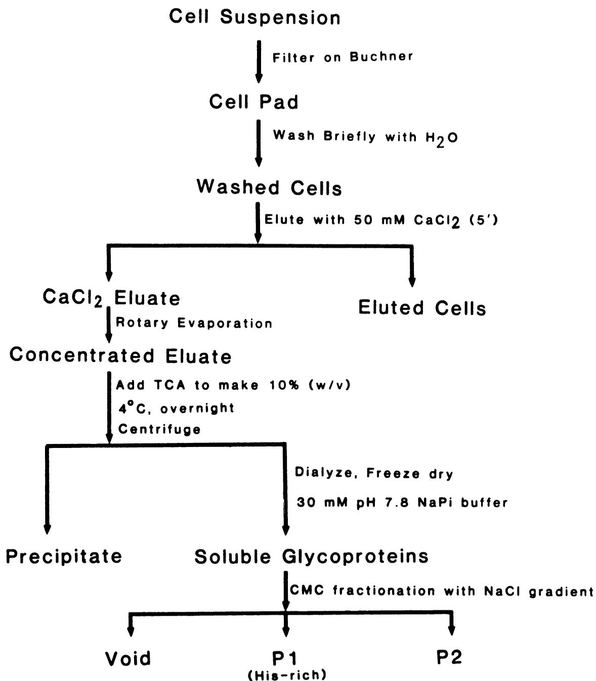
**Figure 3.** Flow chart for bulk elution and purification of hydroxyproline-rich glycoprotein from tomato suspension cultures.
