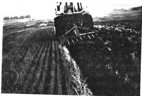
Figure 6.3.19 PTO Driven Disk Tiller Performance in Friable Soil Conditions
