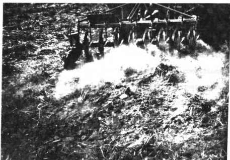
Figure 6.3.17 PTO Driven Disk Tiller Performance in Dry Soil Conditions; Penetration Impaired
