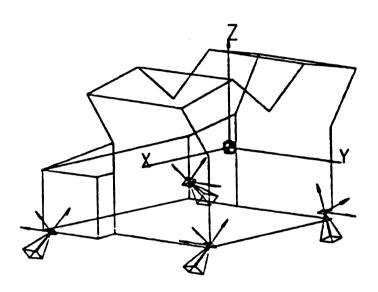
Figure 1 Engine/mounts coordinate system
