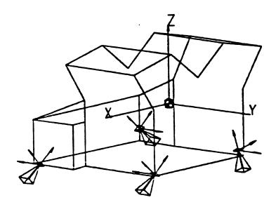
Figure A1 Engine/mounts coordinate system
