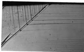
Figure 15. Basal slip traces across (1\bar{1}02)[1\bar{1}0\bar{1}] twin boundary in S.B. No. 5. (10\bar{1}0) edge of specimen F-4. 100 x. (a) P = 4.0 kg (b) P = 4.8 kg.
