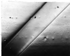
Figure 20. Growth and untwinning of (1\bar{1}02)[1\bar{1}01] twin in S.B. No. 6. (11\bar{2}0) edge of specimen G-4. P = 860 g. 70\times . (a) Growth on tension side. (b) Untwinning on compression side.
