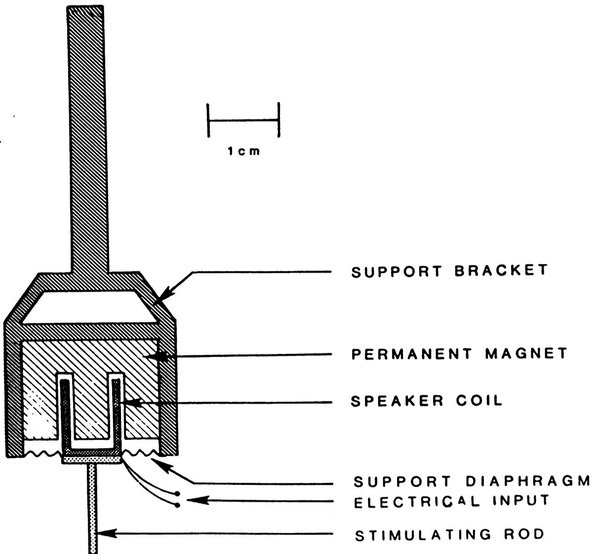
Figure 9. This drawing is a cross section of the mechanical stimulator. Displacements of the stimulating rod were obtained by applying a current pulse to the electrical inputs of the speaker coil.
