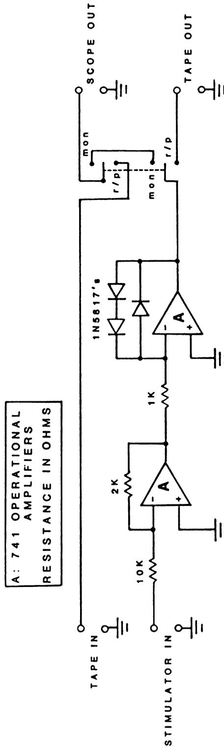
Figure 12. Circuit diagram of the stimulus event marker. Stimulus event marks shown in figures 7 and 13 were provided by the circuit diagrammed in this figure. Parallel output of the voltage source driving the circuit shown in figure 10 provided input to the event marker circuit. Output from this circuit could be switched in order to monitor it directly ("mon") or to record and monitor it from magnetic tape ("r/p").
