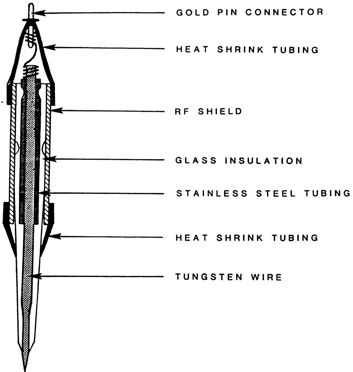
Figure 3. This sketch of the microelectrode for recording unit activity is not drawn to scale. Electrodes varied between 5 and 8 cm in length with uninsulated tips 10-50 $\mu$  in length, and tapering from 10-25 $\mu$  in diameter.
