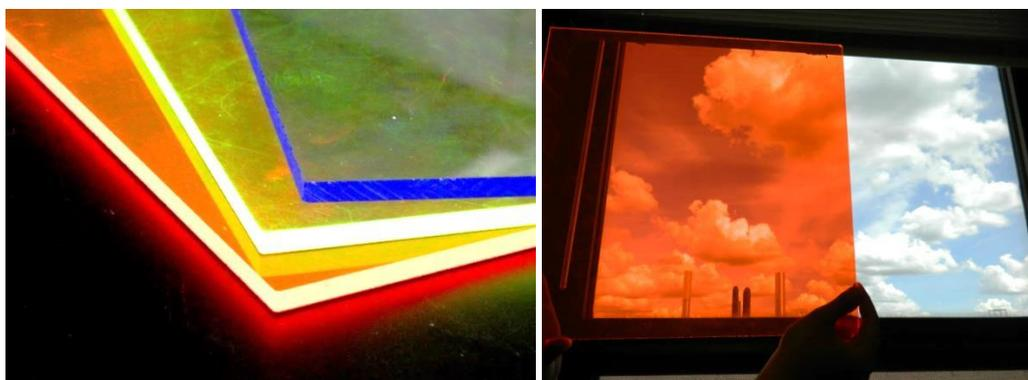
**Figure 2.3** Photograph of typical colorful luminescent solar concentrators highlighting the waveguided emission that is brightly focused at the edge. (b) Example of a traditional LSC in front a window, highlighting the difficulty in installing these systems in a variety of applications such as windows.
