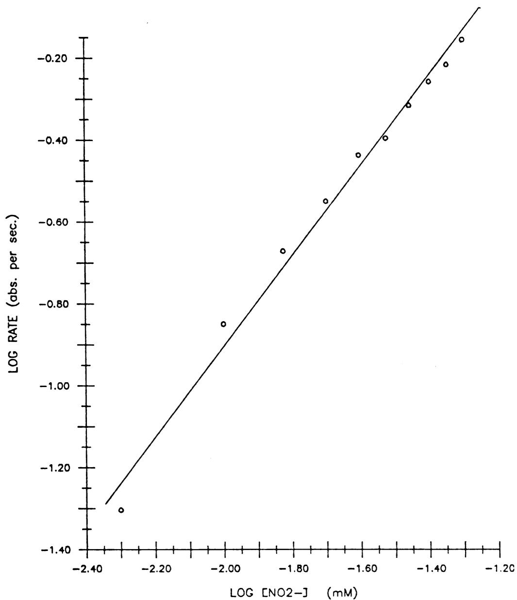
Figure 10. Calculation of order of the diazonium ion formation step due to  $\text{NO}_2^+$ .
