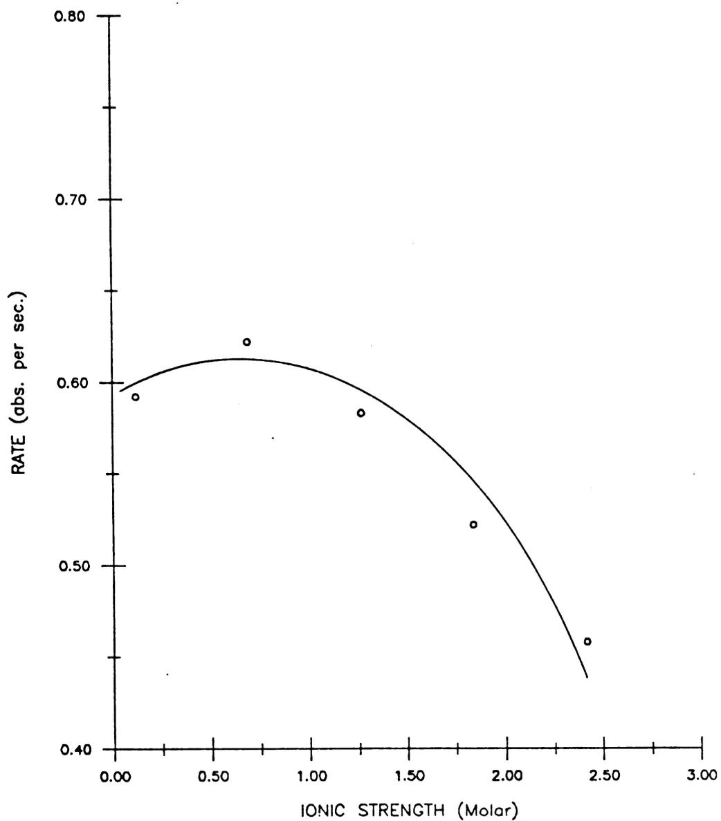
Figure 20. Effect of ionic strength on the coupling reaction.
