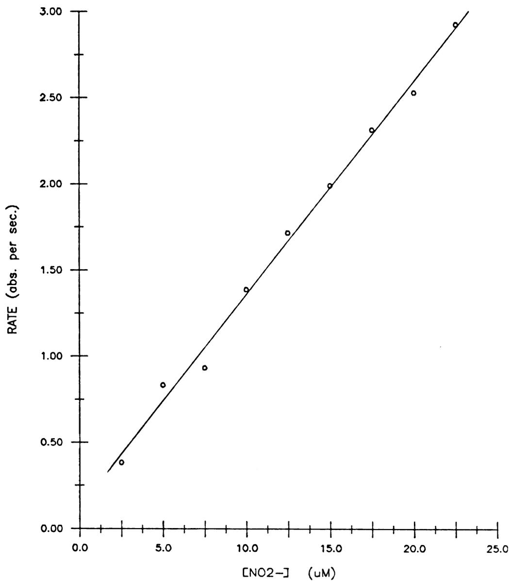
Figure 16. Dependence of rate of the coupling reaction on  $[\text{NO}_2^-]$ .
