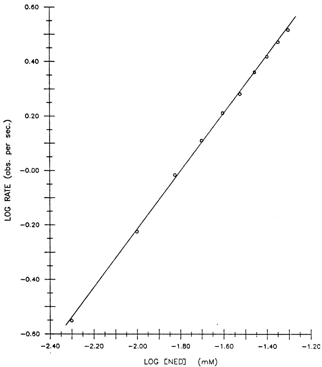
Figure 12. Calculation of order of the coupling step due to NED.
