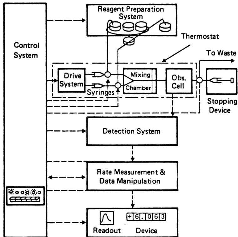
Figure 2. General diagram of stopped-flow system.
