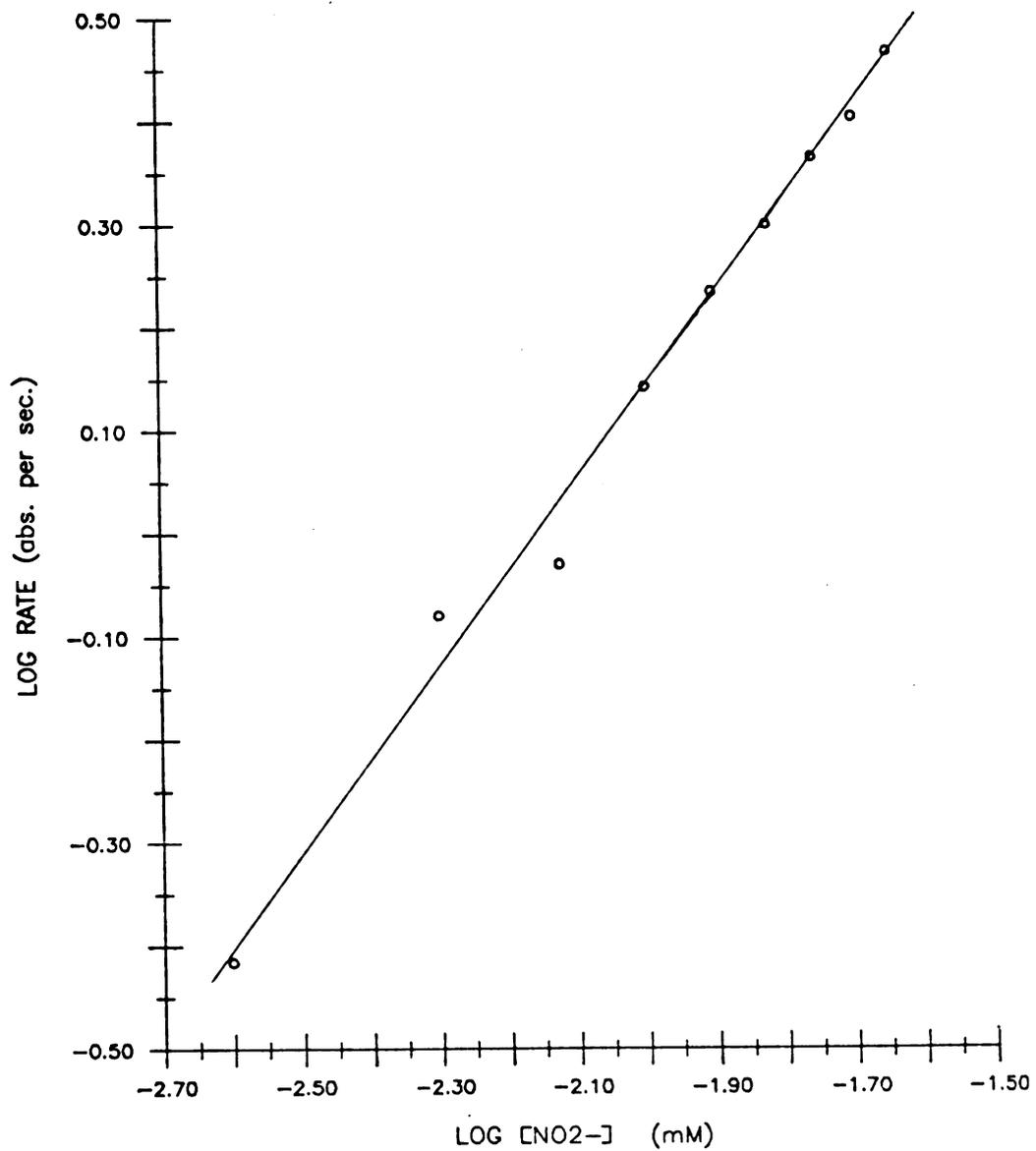
Figure 11. Calculation of order of the coupling step due to  $\text{NO}_2^-$ .
