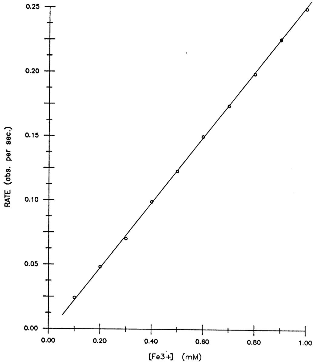
Figure 9. Dependence of rate of the iron-thiocyanate reaction on  $[\text{Fe}^{3+}]$
