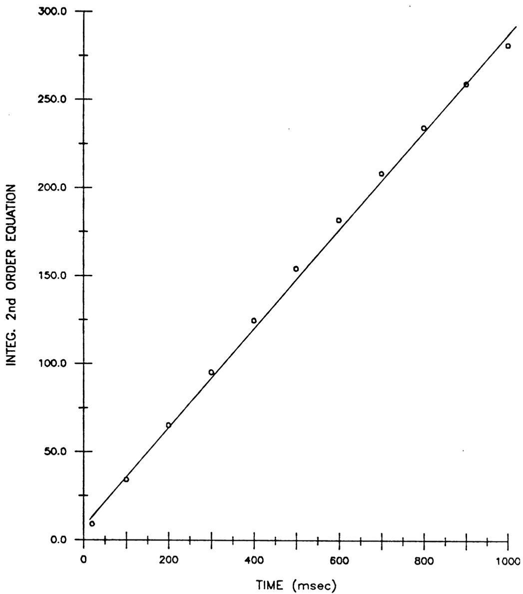
Figure 14. Confirmation of order of the coupling reaction.
