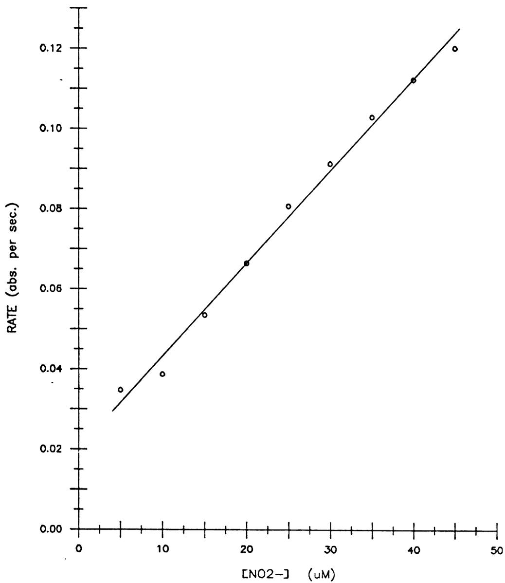
Figure 18. Dependence of the simultaneous reaction rate on  $[\text{NO}_2^-]$ .
