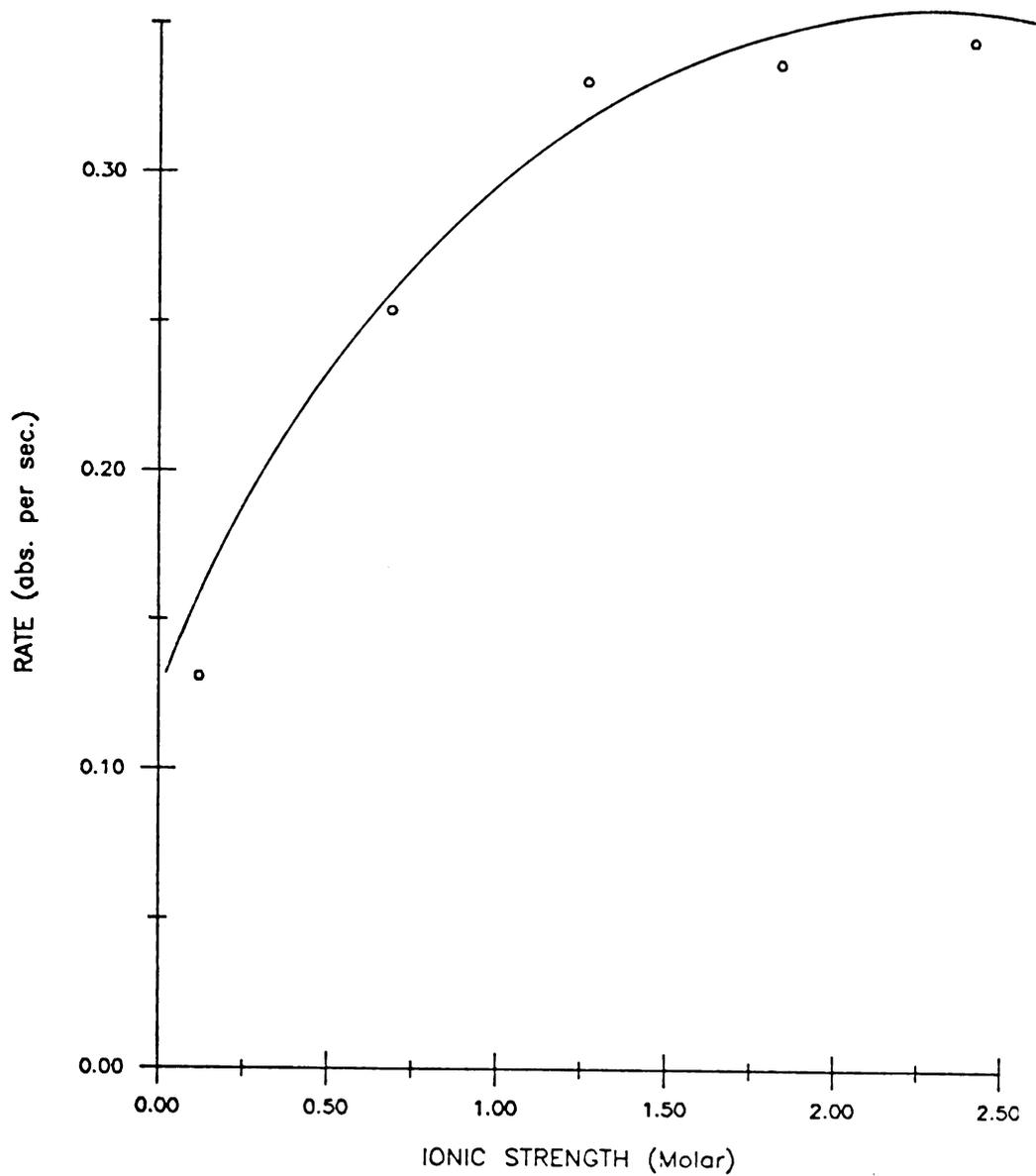
Figure 19. Effect of ionic strength on rate of diazonium ion formation.
