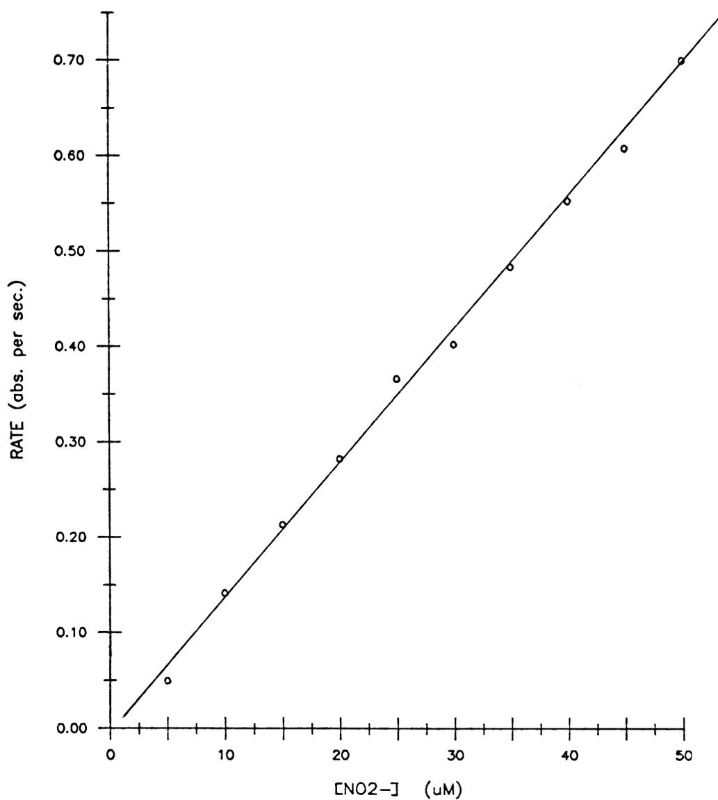
Figure 15. Dependence of the diazonium ion formation rate on  $[\text{NO}_2^-]$ .
