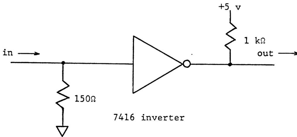
Figure 6. Controller circuit for opto-interrupter.
