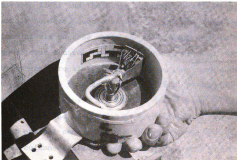
Figure 8: An absolute shaft encoder was used to determine the actual position of the wheels and sensor arms.
