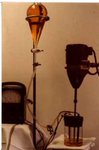
Figure 2. Setup of Emulsion Formation Apparatus Showing from Left to Right, Ohm Meter, Oil Reservoir and Delivery Tubing, "Lightin Mixer" and Beaker.
