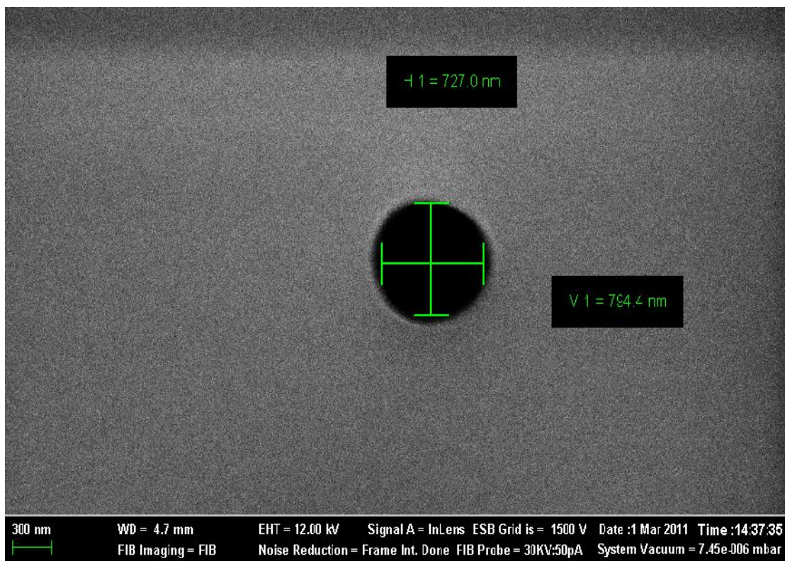
Figure 5.1: SEM image of nanopore on \text{Si}_3\text{N}_4 window. The horizontal (H1) and vertical (V1) diameters are 727.0 nm and 794.4 nm, respectively.
