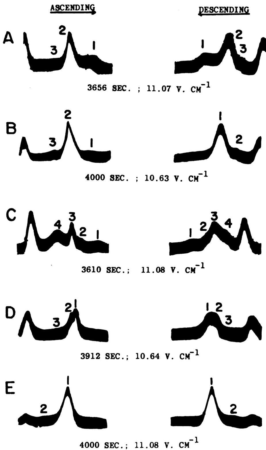
Figure 25. Electrophoretic patterns of (A) proteose-peptone, (B) sigma-proteose, (C) whey component 5, (D) minor-protein fraction and (E) soluble membrane protein. The fractions were run in veronal buffer, pH 8.6,  $\Gamma/2 = 0.1$  at 1.5% concentration.
