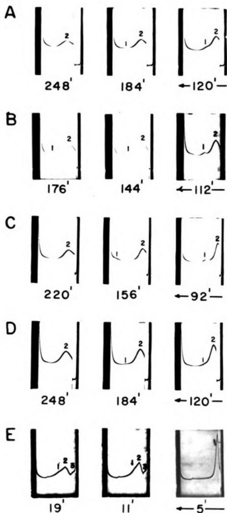
Figure 27. Sedimentation diagrams in veronal buffer, pH 8.6,  $\Gamma/2 = 0.1, 1, 5\%$  concentration of (A) proteose-peptone, (B) sigma-protease, (C) whey component 5, (D) minor-protein fraction and (E) soluble membrane protein. All phase plate angles were at  $60^\circ$ . Rotor speeds for A-D were 59,780 r.p.m. and E. was 52,640 r.p.m.
