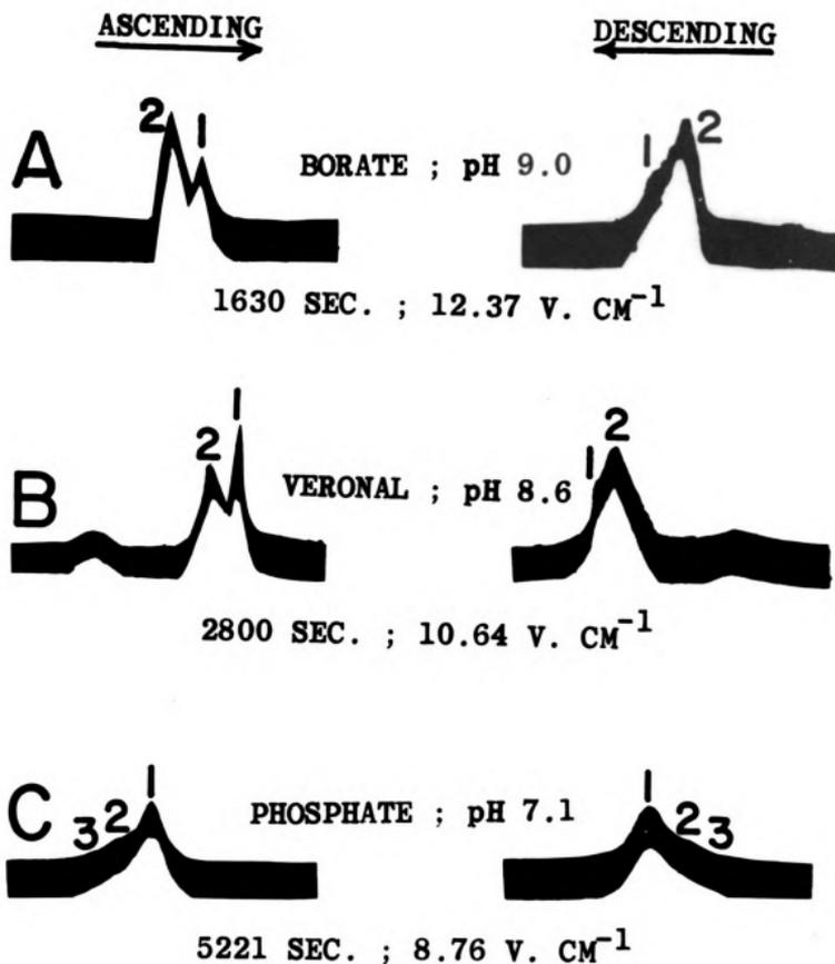
Figure 38. Electrophoretic patterns of NaCl fractionated lipoproteins at approximately 0.75% concentration in buffers indicated. (A) was run at  $\Gamma/2 = 0.05$ , (B) and (C) at  $\Gamma/2 = 0.1$ .
