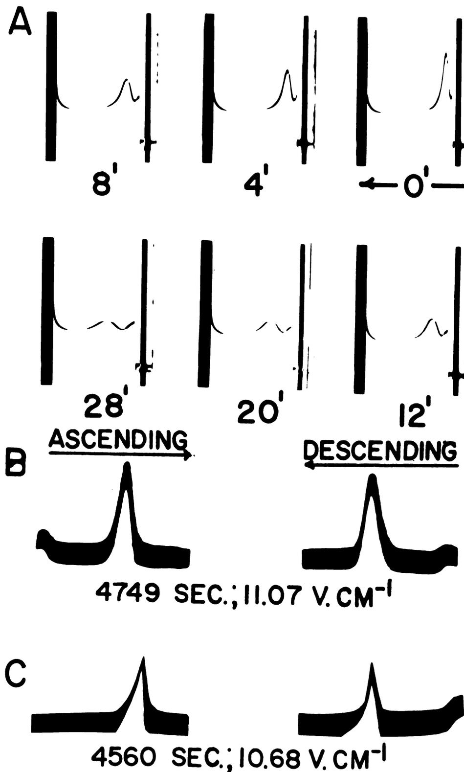
Figure 33. (A) and (B) represent ultracentrifugal and electrophoretic analyses of the lipid-free protein obtained from sucrose fractionated membrane sera. The protein concentrations for (A) and (B) were 0.70 and 1.0%, respectively. (C) represents the electrophoretic pattern of the native insoluble membrane protein at 0.5% concentration. All fractions were studied in veronal buffer, pH 8.6,  $\Gamma^2/2 = 0.1$ .
