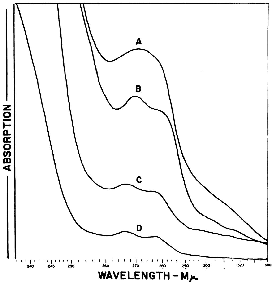
Figure 10. Ultraviolet spectra of ethanol extracts of the high-melting glyceride. Curve A, first extract, diluted 1:2, 0.1 cm. path. Curve B, second extract, diluted 1:1, 0.1 cm. path. Curve C, third extract, undiluted, 0.1 cm. path. Curve D, fourth extract, undiluted, 1.0 cm. path.
