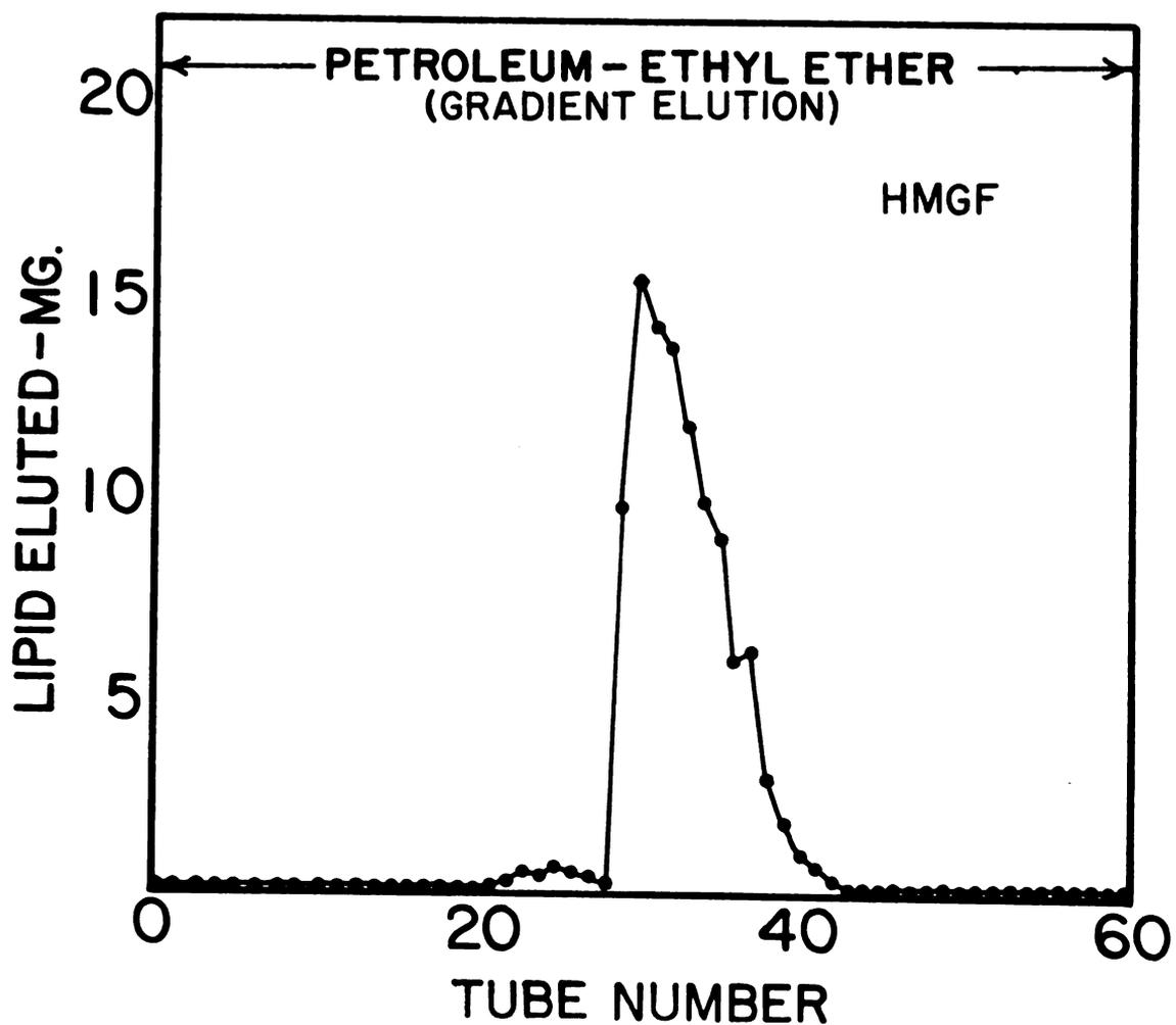
Figure 15. The separation of the high-melting glyceride fraction by elution from an 18 g. column of silicic acid. Ten percent ethyl ether was employed in the top reservoir with a lipid charge of 108.3 mg.
