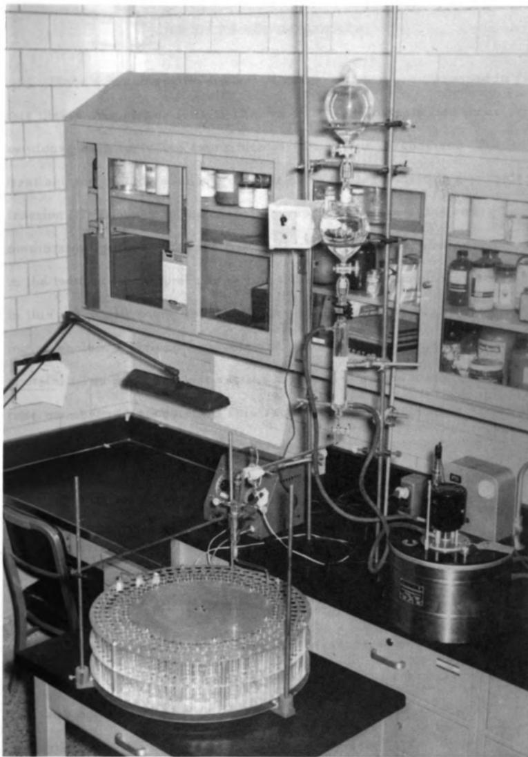
Figure 9. Photograph of equipment employed in silicic acid chromatography of membrane and butteroil fractions.
