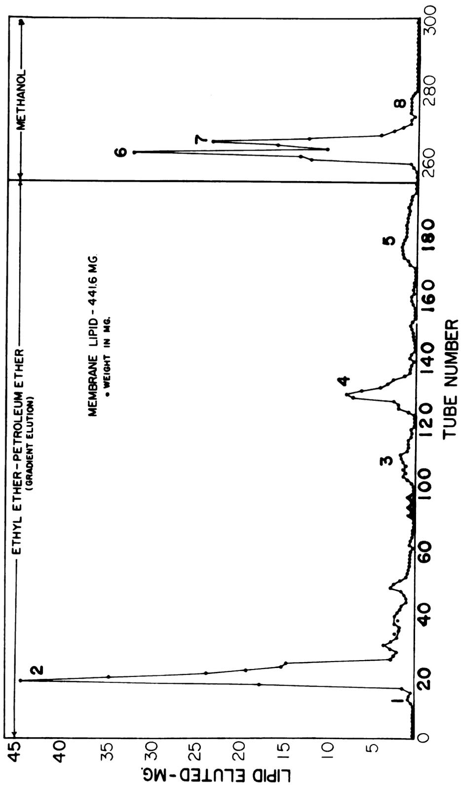
Figure 22. The separation of lipid components from the milk fat-globule membrane (scheme I) eluted from an 18 g. column of silicic acid. Lipid charge was 280.0 mg.
