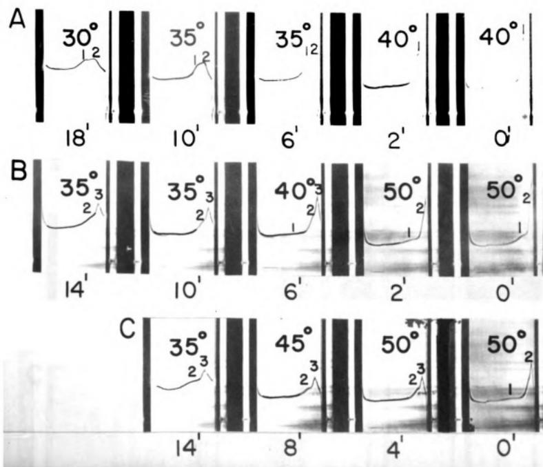
Figure 35. Ultracentrifugal diagrams of membrane lipoproteins fractionated with sodium chloride. (A), (B) and (C) represent analysis in water, veronal buffer at pH 8.6,  $\Gamma/2 = 0.1$  and veronal buffer at pH 8.6,  $\Gamma/2 = 0.05$  respectively.
