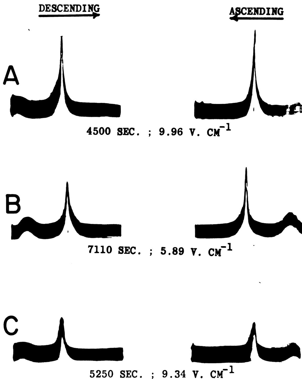
Figure 31. Electrophoretic patterns of insoluble membrane proteins solubilized with (A) basis solution, (B) 3% peracetic acid and (C) 2' thiodiethanol at concentrations of 0.60, 0.53, and 0.40% respectively. The fractions were run in veronal buffer, pH 8.6,  $\Gamma/2 = 0.1$ .
