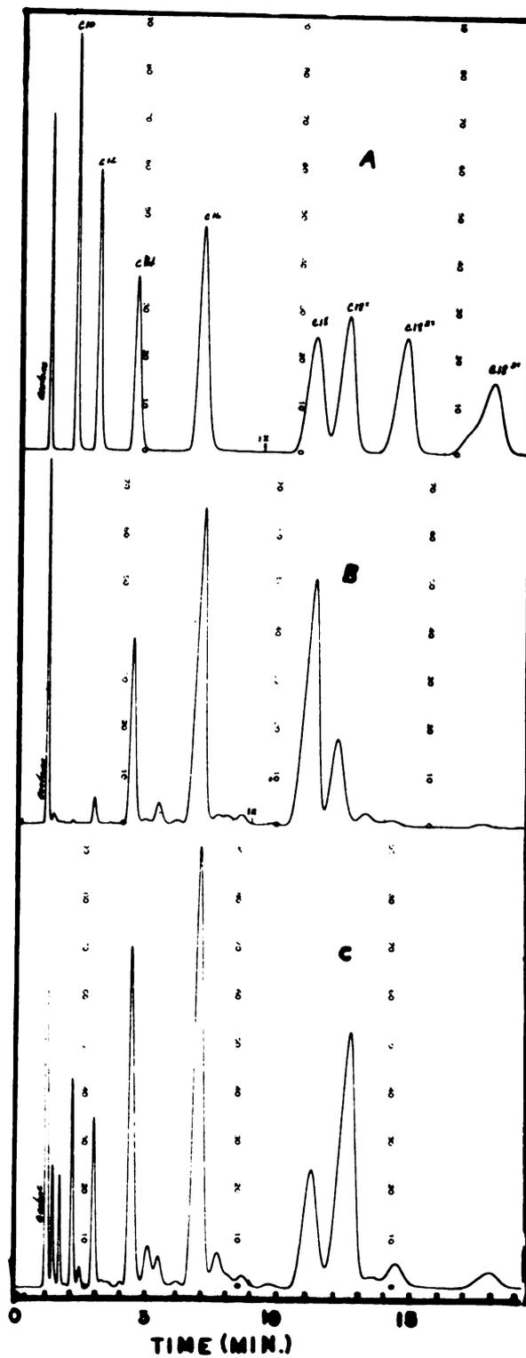
Figure 14. Gas chromatograms of the fatty acid methyl esters of (A) a known mixture of fatty acids, (B) the fat-globule membrane HMGF, and (C) butteroil. 1x denotes time of a twofold increase in detector sensitivity.
