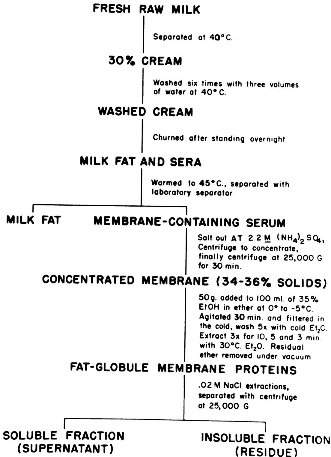
Figure 1. Schematic isolation procedure for obtaining the insoluble and soluble membrane proteins according to Herald (1956).
