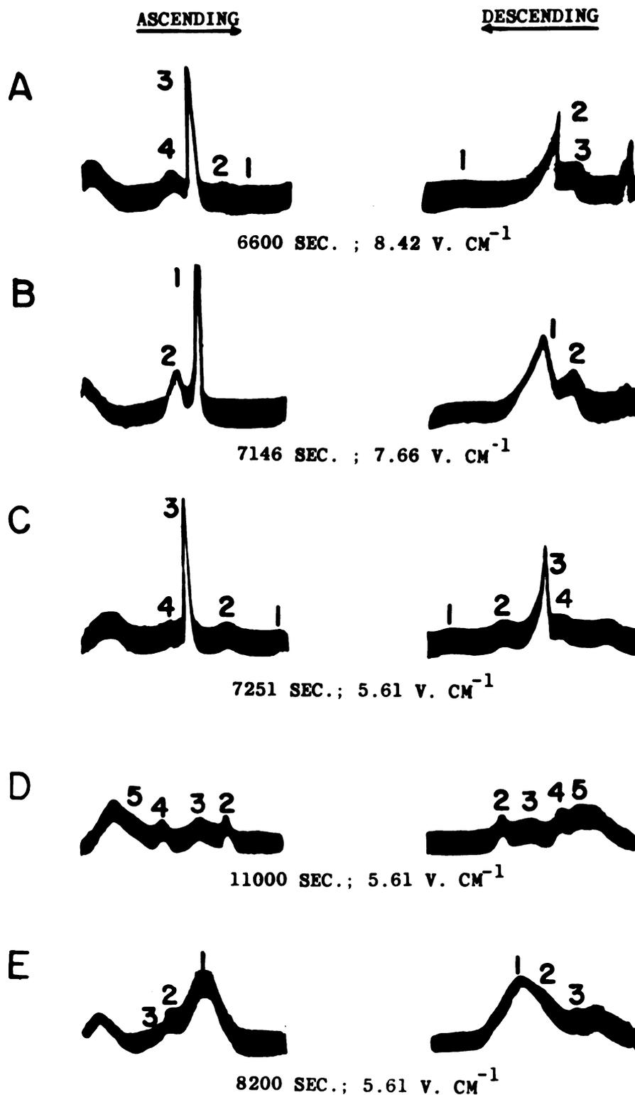
Figure 26. Electrophoretic patterns of (A) proteose-peptone, (B) sigma-protease, (C) whey component 5, (D) minor-protein fraction and (E) soluble membrane protein. The fractions were run in HCl-NaCl buffer, pH 2.4,  $\Gamma/2 = 0.1$  at 1.5% concentration.
