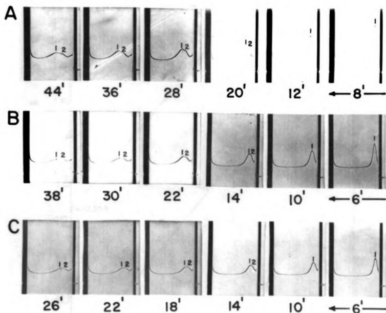
Figure 36. Ultracentrifugal diagrams lipid-free proteins obtained by ethanol-ether extraction of the sucrose fractionated lipo-protein. Protein concentrations are 1.5% for (A), 1.0% for (B), and 0.75% for (C). The buffer system was veronal at pH 8.6,  $\Gamma/2 = 0.1$ . The rotor was operated at 52,640 r.p.m. with the phase plate maintained at  $60^\circ$ .
