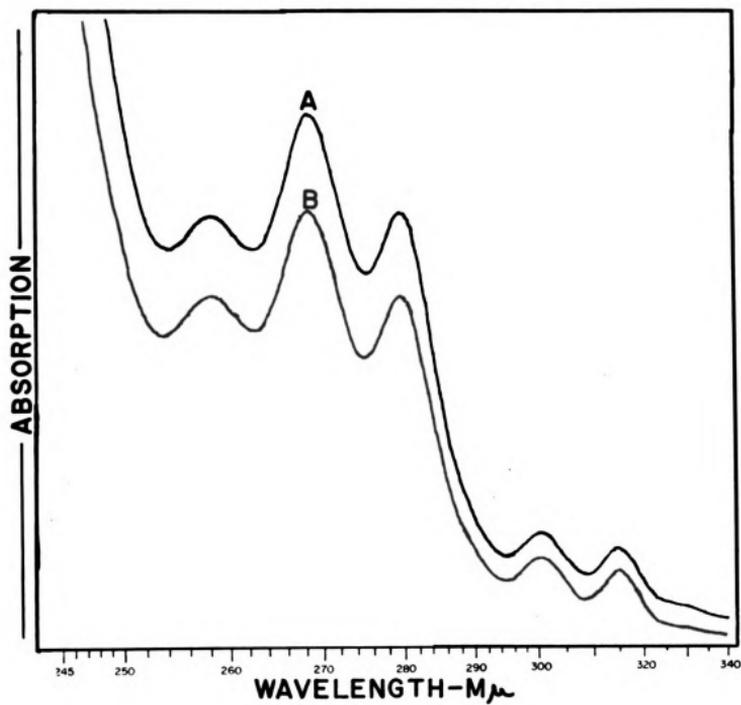
Figure 11. Ultraviolet absorption spectra of the high-melting glyceride fractions obtained from (A) butteroil and (B) the fat-globule membrane.
