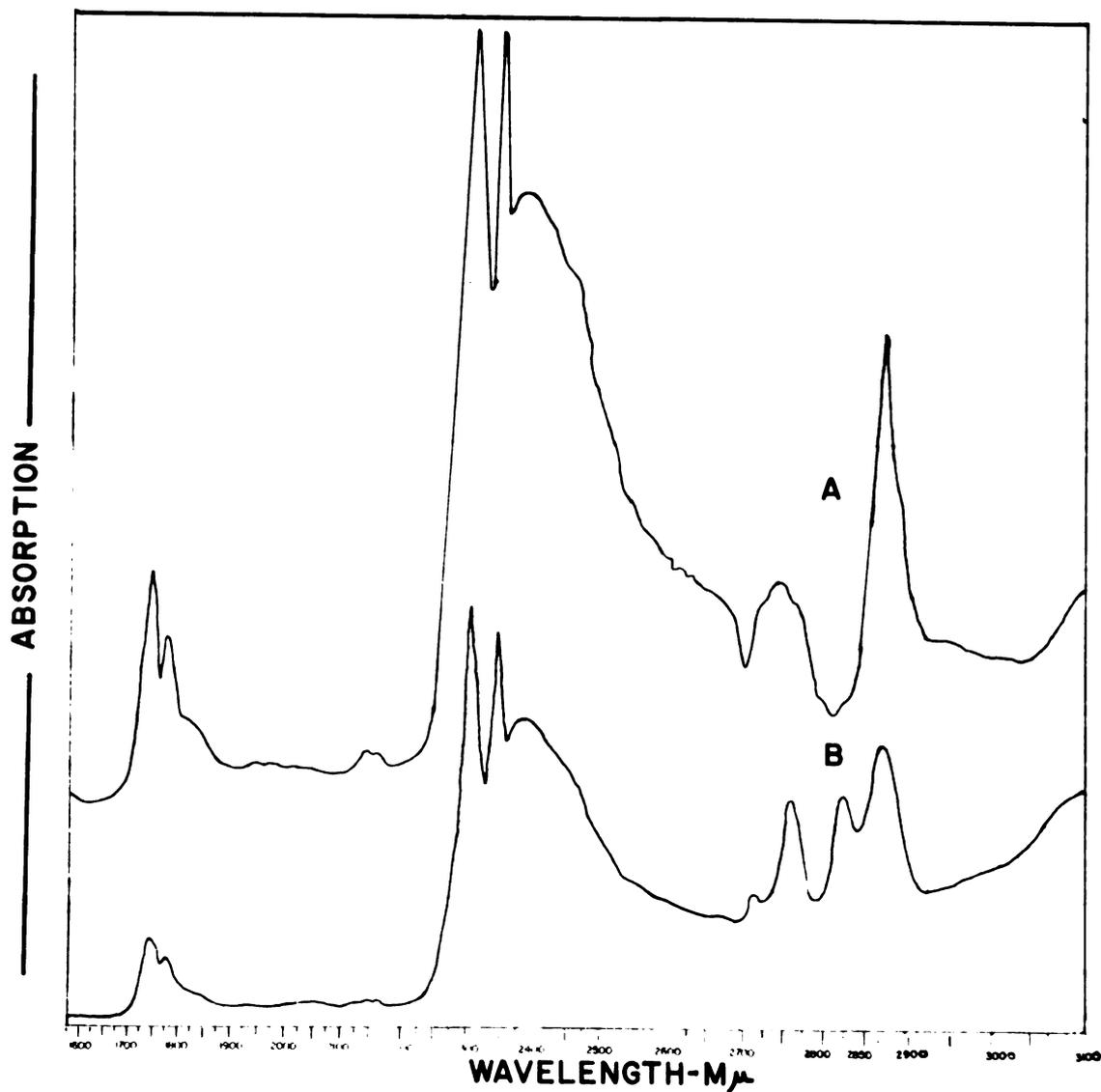
Figure 12. Near-infrared (photoelectric) absorption spectra of (A) tristearin and (B) the high-melting triglyceride in  $\text{CCl}_4$ . Concentrations approximate 5%.
