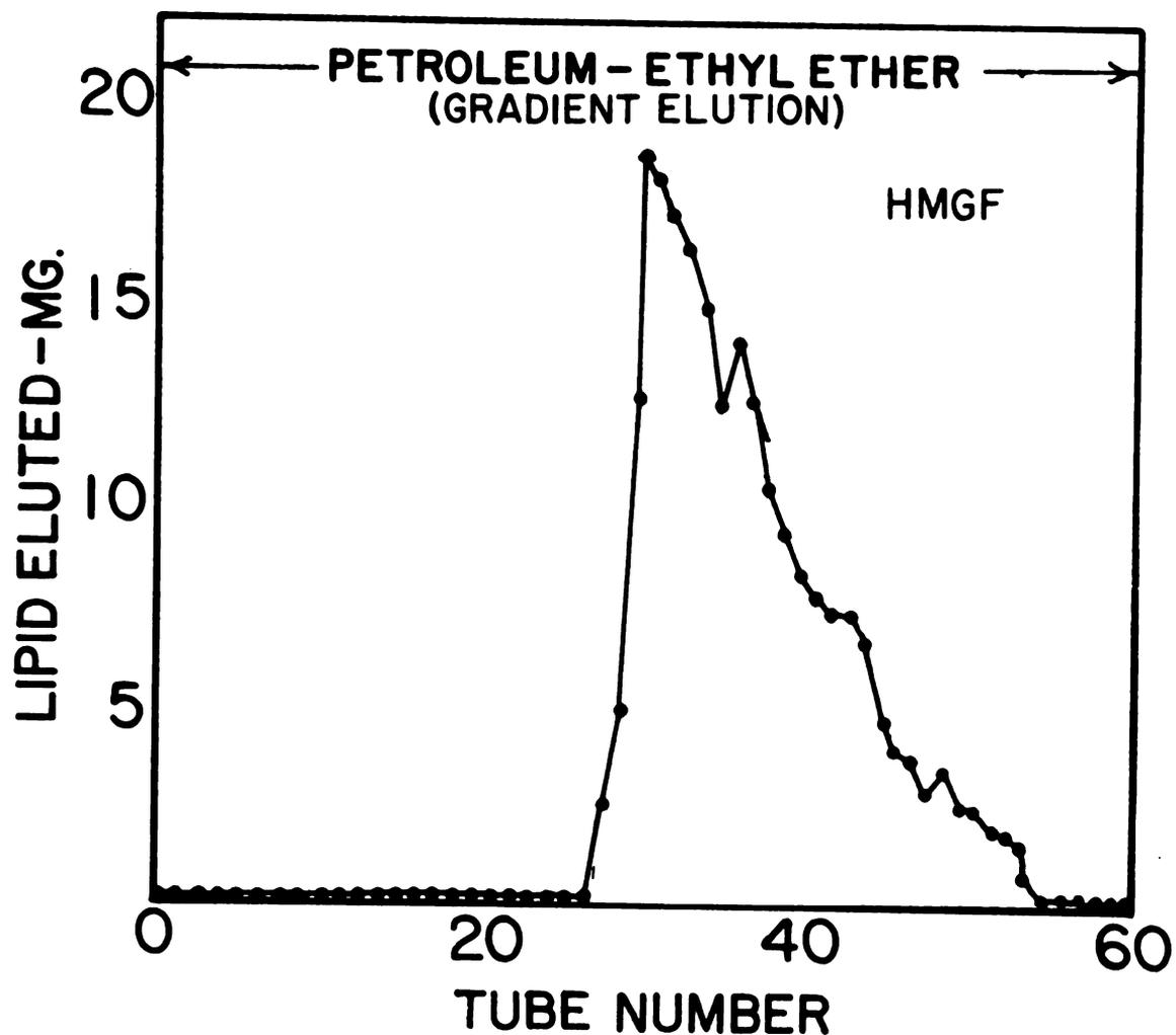
Figure 16. The separation of the high-melting glyceride fraction by elution from an 18 g. column of silicic acid. Five percent ethyl ether was employed in the top reservoir with a lipid charge of 305.1 mg.
