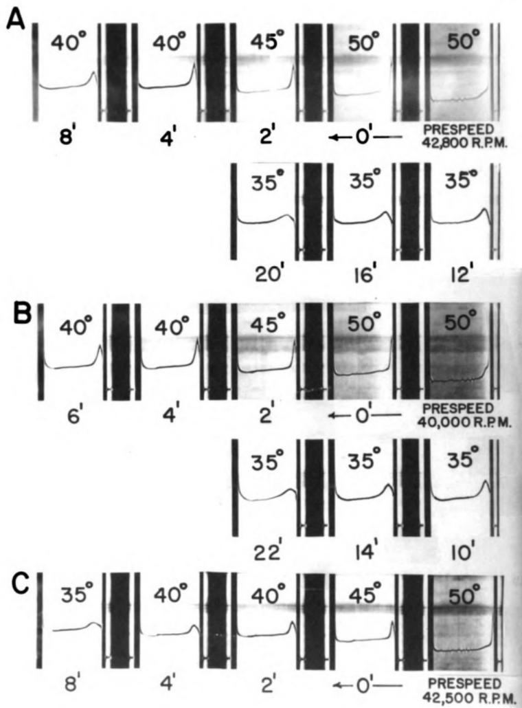
Figure 39. Ultracentrifugal diagrams of salt fractionated lipoproteins in (A) borate buffer,  $\Gamma/2 = 0.05$ , (B) veronal buffer, and (C) phosphate buffer at  $\Gamma/2 = 0.1$ .
