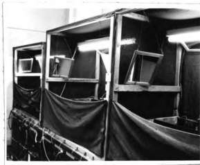
Figure 4. Photograph of Experimental Tanks (external view). This view shows the position of the wooden frame around each Experimental Tank. Blue denim cloth was placed over the frame on the top, back, and both sides. The removable curtain across the front of the frame isolated the fish visually from persons walking past. Mirrors were positioned above each Experimental Tank at a 45° angle in order to observe the fish without disturbing them.
