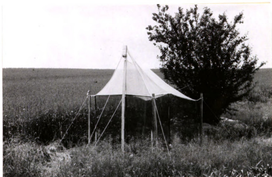
Figure 31. Type of malaise trap used to monitor flight activity of Diaparsis n.sp.
