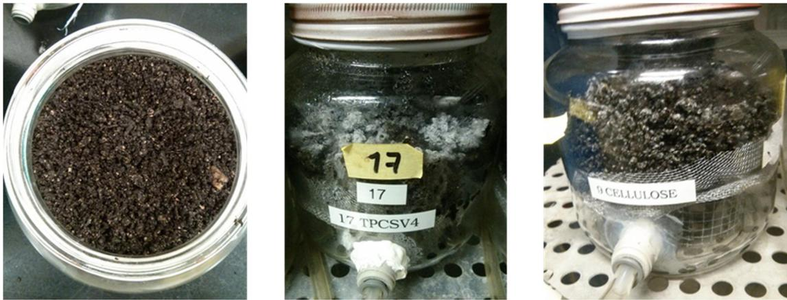
Figure 4.5 Biodegradation of thermoplastic cassava starch reinforced by natural fiber in DMR system
